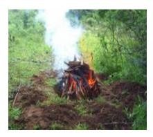
between preparing in a pit and open space is that charcoal prepared in the pit burns gradually and gives heat for a long time, while charcoal prepared on the surface is used for shorter time periods.
