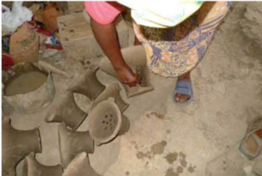
Figure 5. The potter demonstrating how a coal pot is smoothed with a polishing stone.
