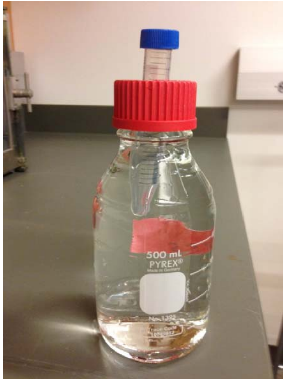
Figure 2.1 “Piston Bottle” for minimization of headspace during heating and cooling
