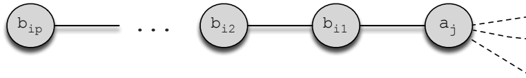
Figure 3.6. Extended clause gadget, C'_j , used in Section 3.3.6. All nodes are injection nodes.
