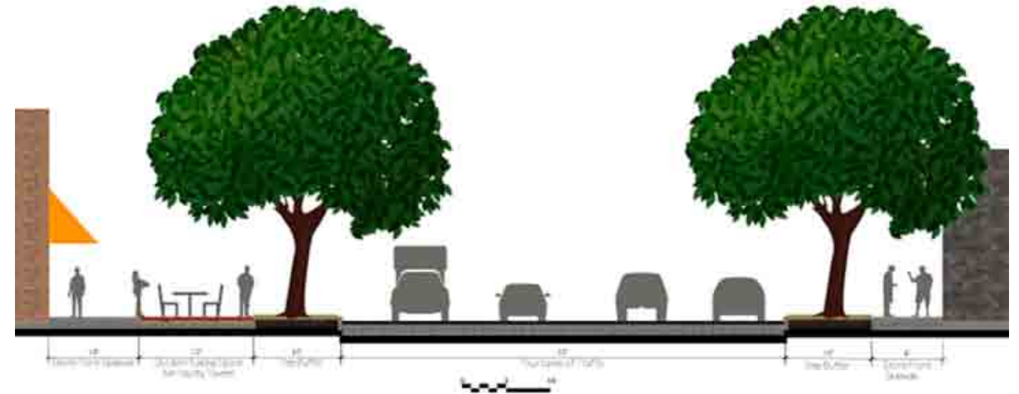
The redesign of same area shifts the emphasis away from the automobile and allows for a more pedestrian friendly environment. Added spaces for water to infiltrate and street trees will help reduce stormwater overflows.
