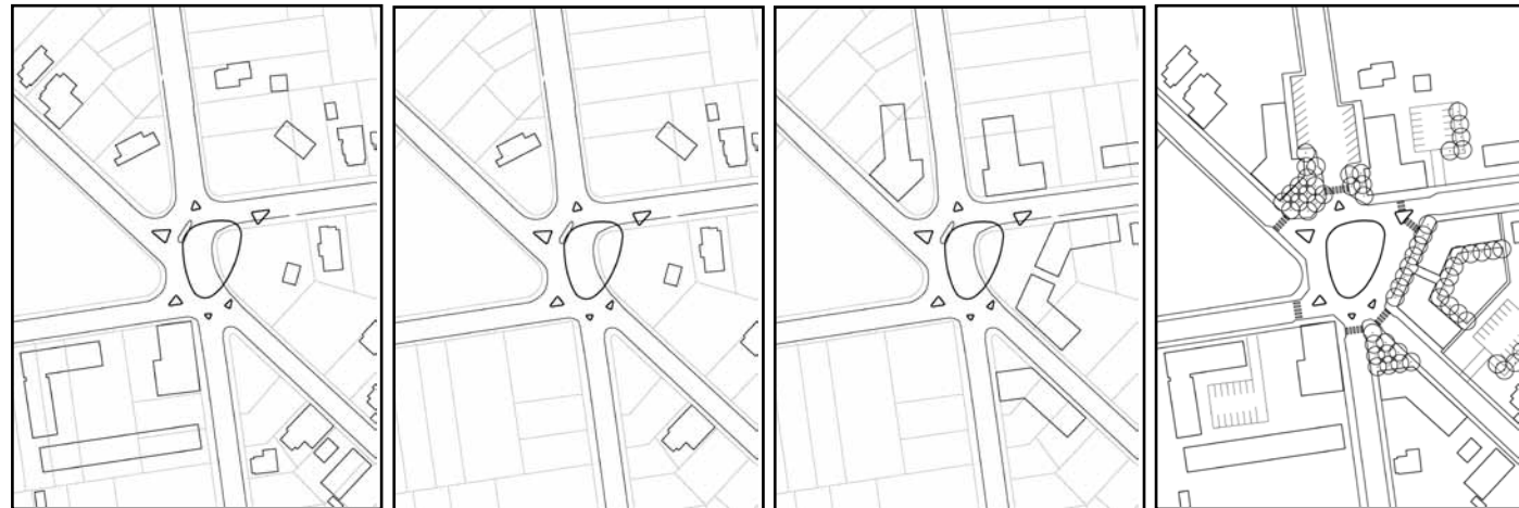
Roundabout, adding nearly one third acre pervious surface.
