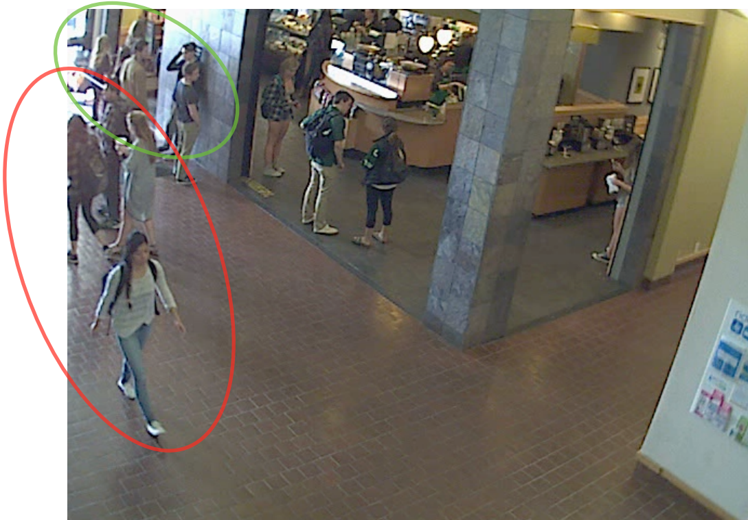
Figure 4.1: Example of the four noise sources. The green circle is stationary people in line. These targets have a perspective change due to camera position, they are overexposed due to lighting coming from the upper left corner, and they are subject to extreme occlusion. The red circle is people in motion. These people walk in front of the stationary targets. not only causing further occlusion, but also challenges for any background subtraction techniques
