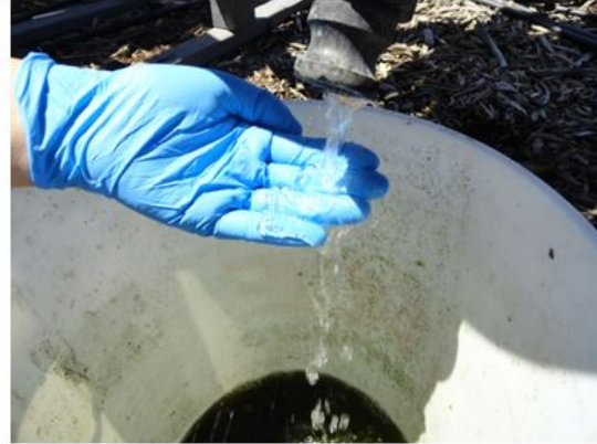
Figure 3-22: Accumulated solids were being drained from the bottom of the tube settlers. The left image illustrates the thick effluent sludge, and the right image illustrates clear water coming through the underdrain after the sludge was removed (Chang, 2014).
