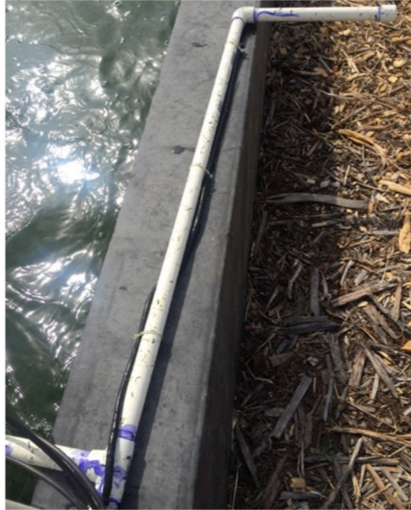
Figure 3-20: Carbon dioxide was sparged into raceways ponds through a black perforated tubing, attached to a PCV stand, that spanned the width of the channel 90 cm downstream of the paddle wheel. It was located on the surface of the pond floor and secured by a weighted PVC pipe. For the image shown the set up was removed from the pond (Kraetsch, 2015).
