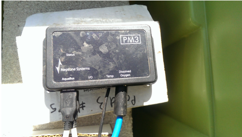
Figure A-3: A Neptune PM3 control unit for DO and temperature data recording. This setup was the same for all ponds (Chang, 2014).
