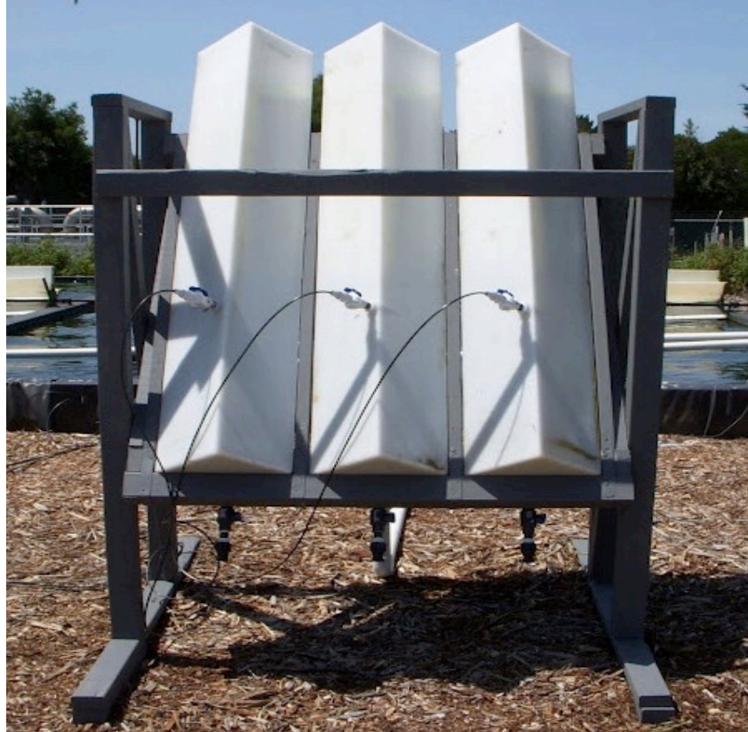
Figure 3-15: Front view of three tube settlers at the AFS. The influent water lines are shown entering the front, and effluent sludge is drained from the valves placed at the bottom (Ripley, 2013).
