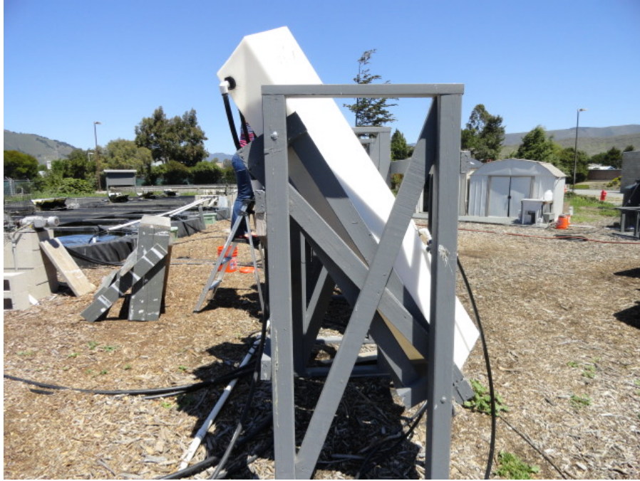
Figure 3-14: Profile view of a tube settler at the AFS. Effluent water from the Round-1 ponds entered the tube settler through the black tubing on the right of the device and exited through the black tubing located at the top left of the device (Chang, 2014).
