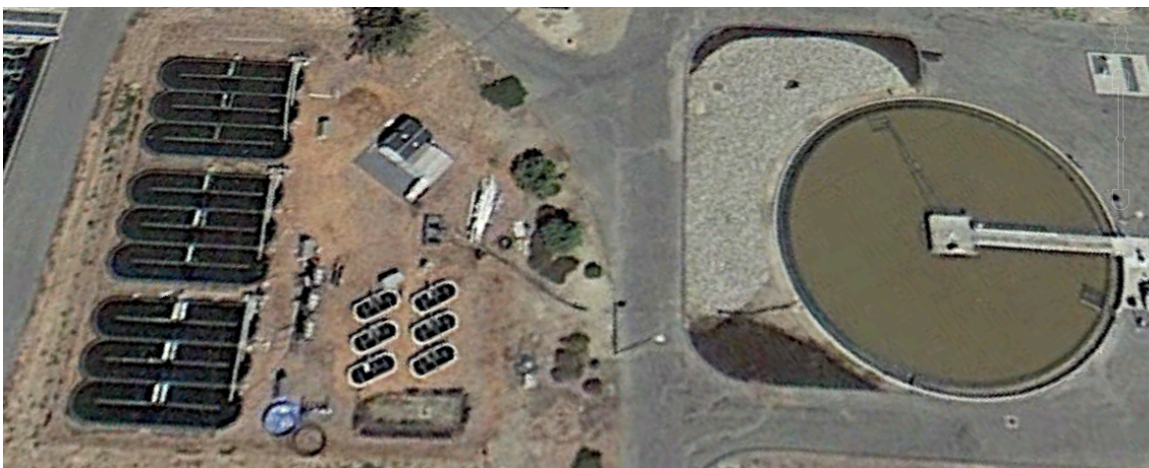
Figure 3-1: Aerial view of the Cal Poly Algae Field Station. The 9 raceway ponds featured in this study are arranged on the left of the image and the source of clarified municipal wastewater was the primary clarifier's effluent water on the right of the image.
