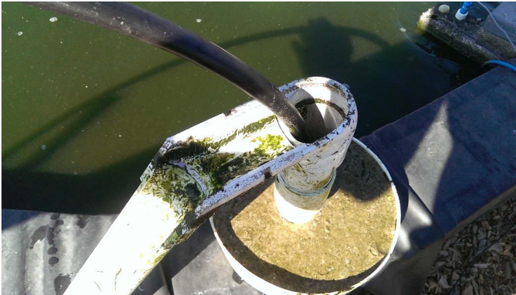
Figure 3-12: Closed bottom ramped standpipe with inserted peristaltic pump tubing for collection of effluent water (Kraetsch, 2015).
