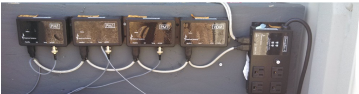
Figure A-2: The Neptune PM1 control units for pH data recording. This setup was the same for all triplicate pond sets (Chang, 2014).
