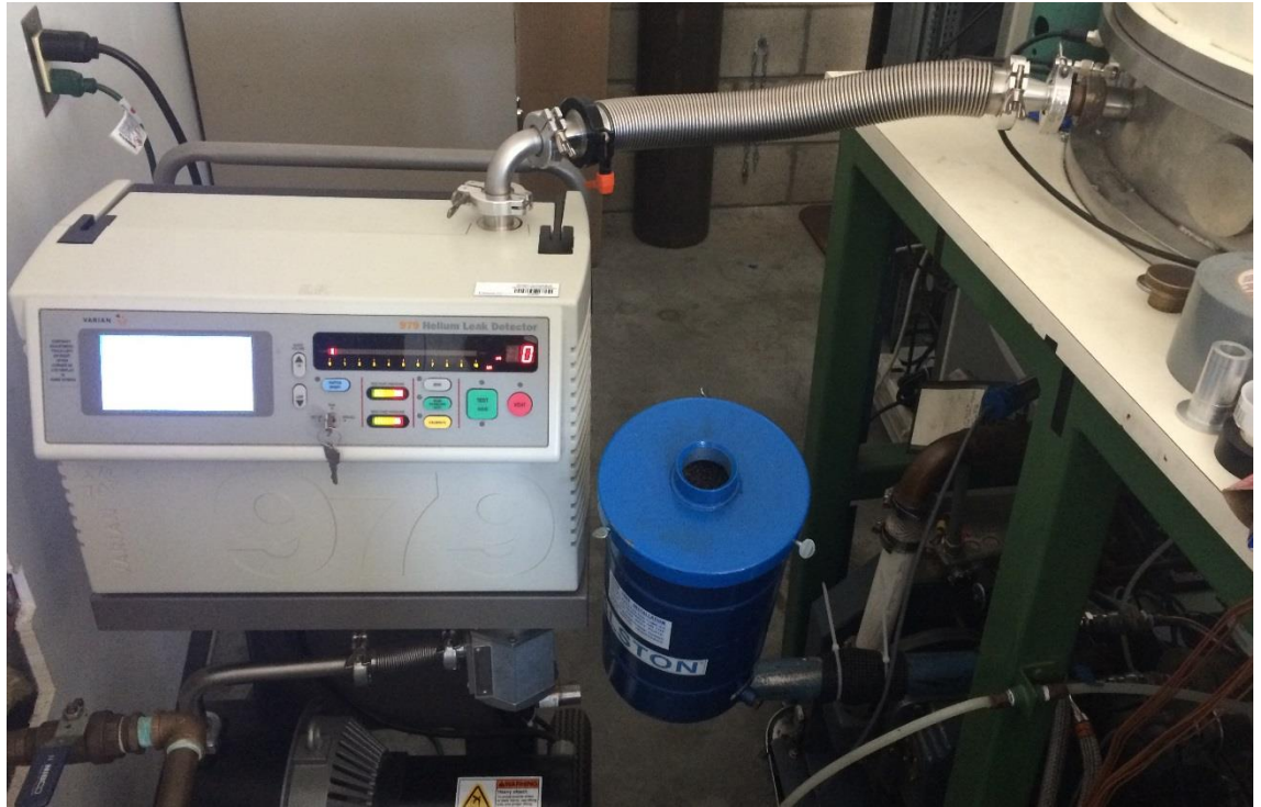
Figure 39. Leak Detector Connected to Vacuum Chamber.
