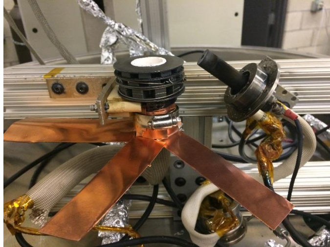
Figure 5. Image of HEMPT and Hollow Cathode. The HEMPT is shown on the left and the hollow cathode is on the right.
