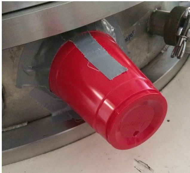
Figure 42. Improved Helium Enclosure Over Area of Suspected Leak. A hole is placed at the bottom of the cup to provide a means of filling the cup with helium.
