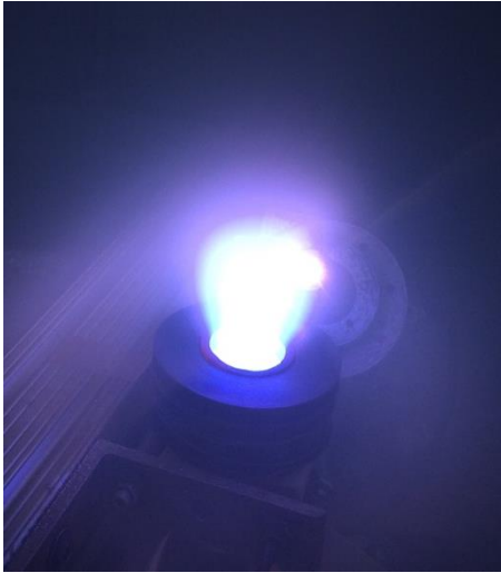
Figure 32. Unshielded HEMPT in Operation.
