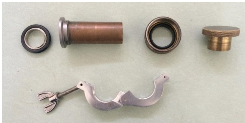
Figure 40. Components Needed for Connecting Leak Detector to Chamber. From upper left to bottom: O-ring, Chamber Port Flange Insert, Brass Backing, End Cap, O-ring Clamp.
