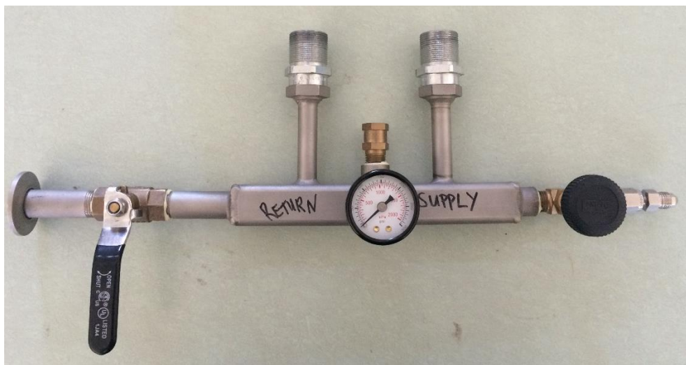
Figure 38. Helium Purge Manifold.
