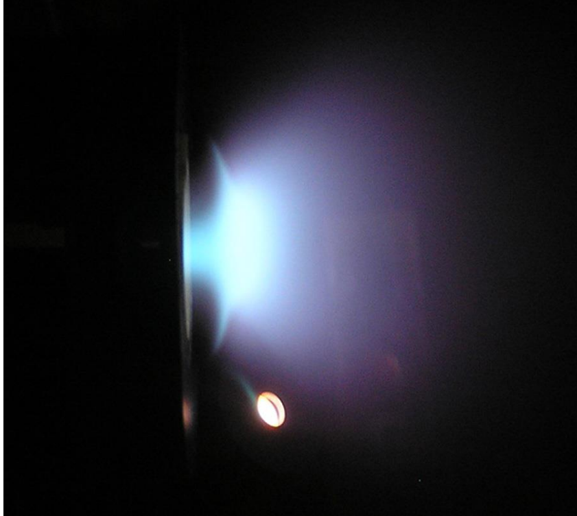
Figure 6. Side view of HEMPT during operation at JPL [7].
