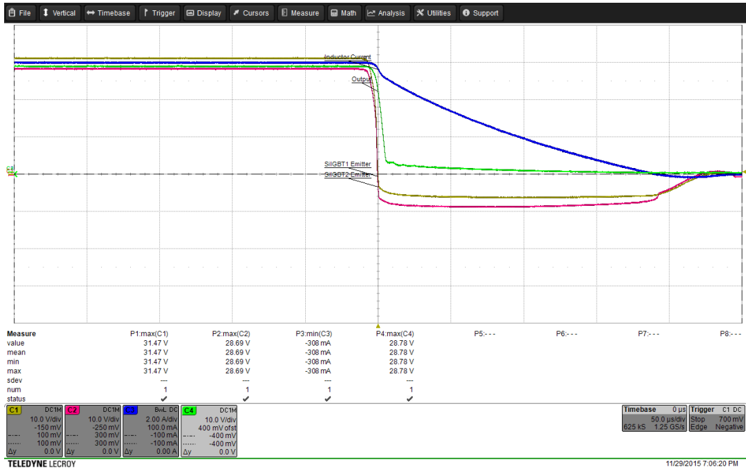
Figure 5-21. Si Breaker Electronic Load Test Results for Zero Output Cap
