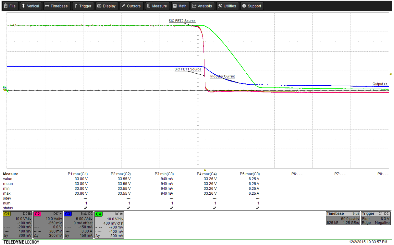
Figure 5-31. SiC Electronic Load Test Result
