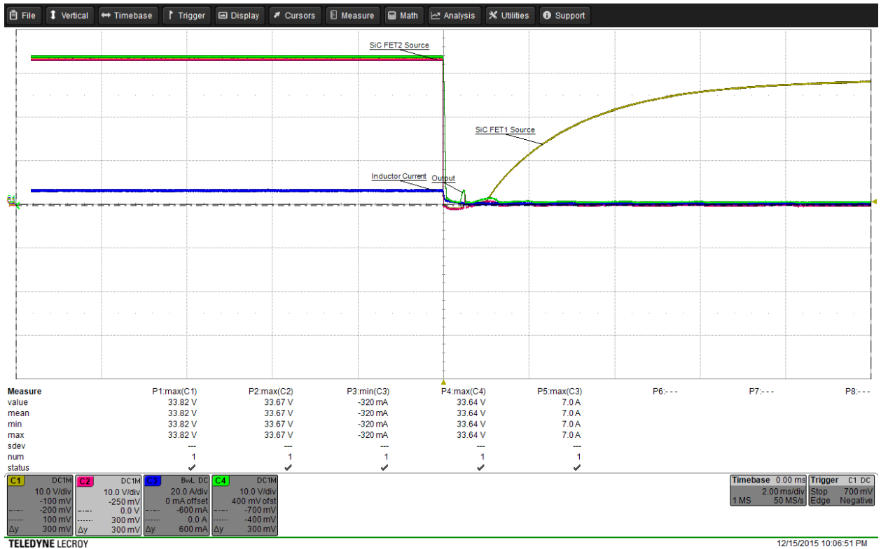
Figure 5-43. SiC FET Electronic Load Test for Modified Driver
