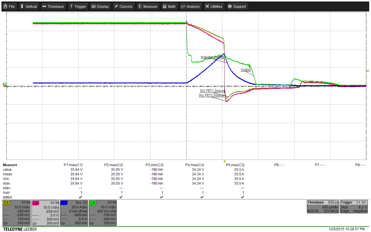
Figure 5-33. SiC Breaker Line Fault Test Result
