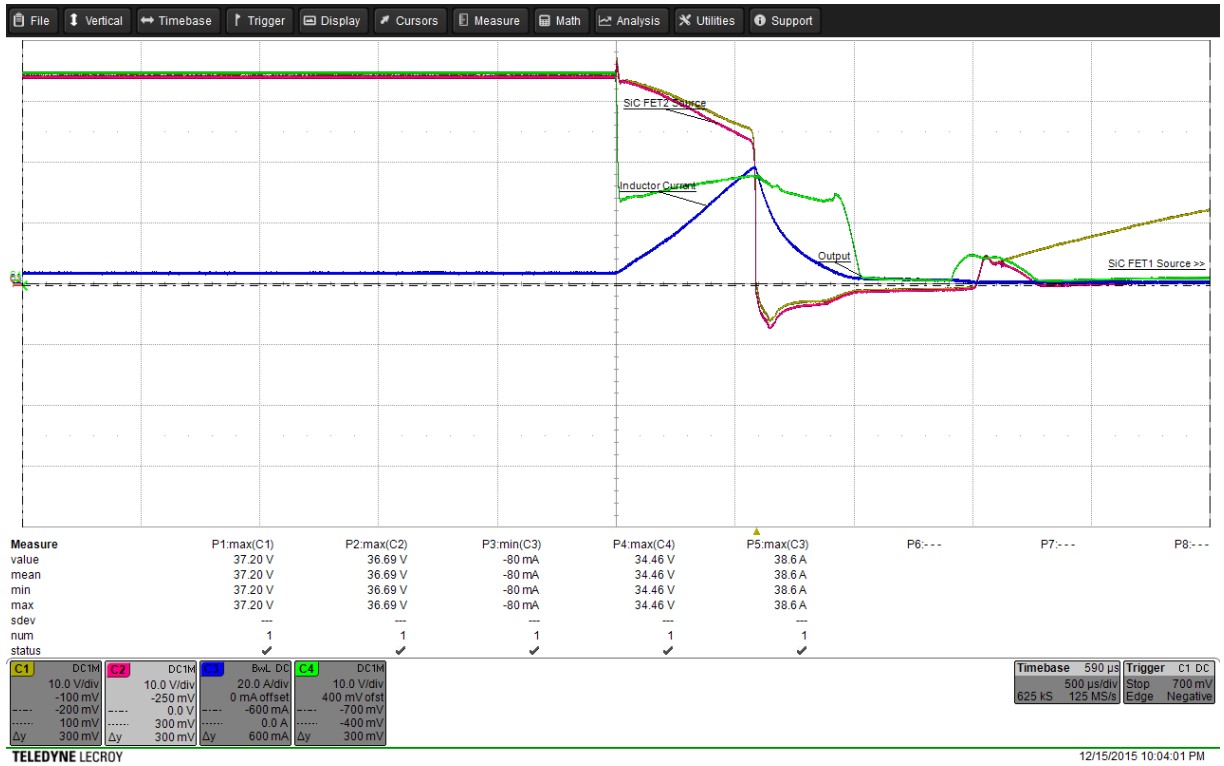
Figure 5-45. SiC FET Line Fault Test for Modified Driver – Response Time
