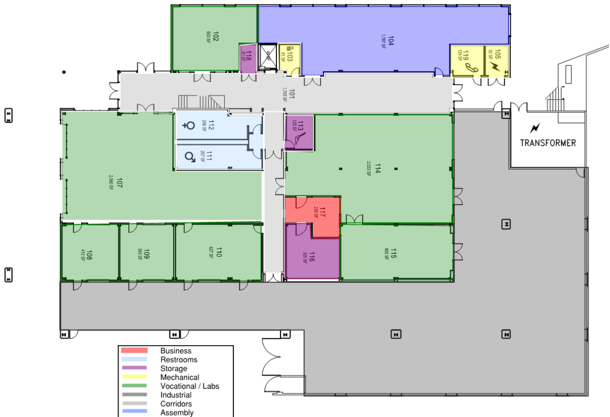
Figure 10 First Floor Occupancy Classification Map
