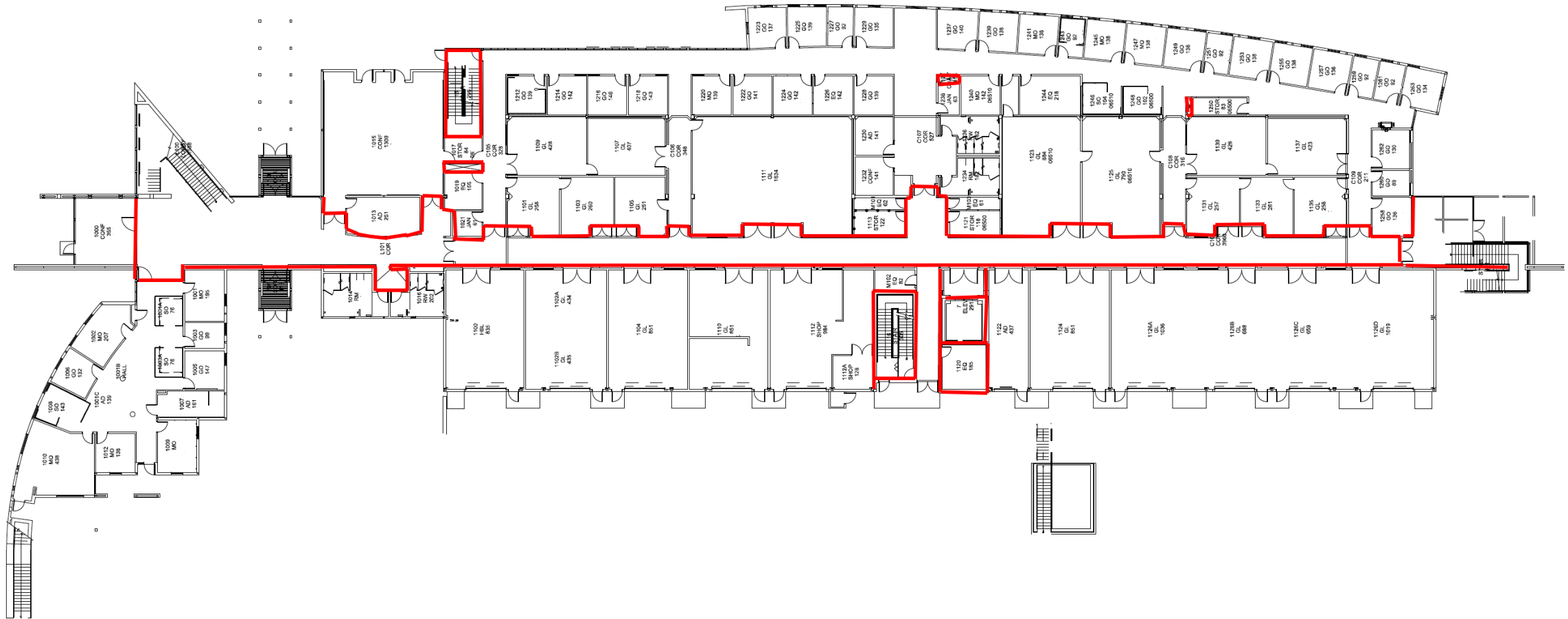
Figure 5-2. First floor fire rated barriers
