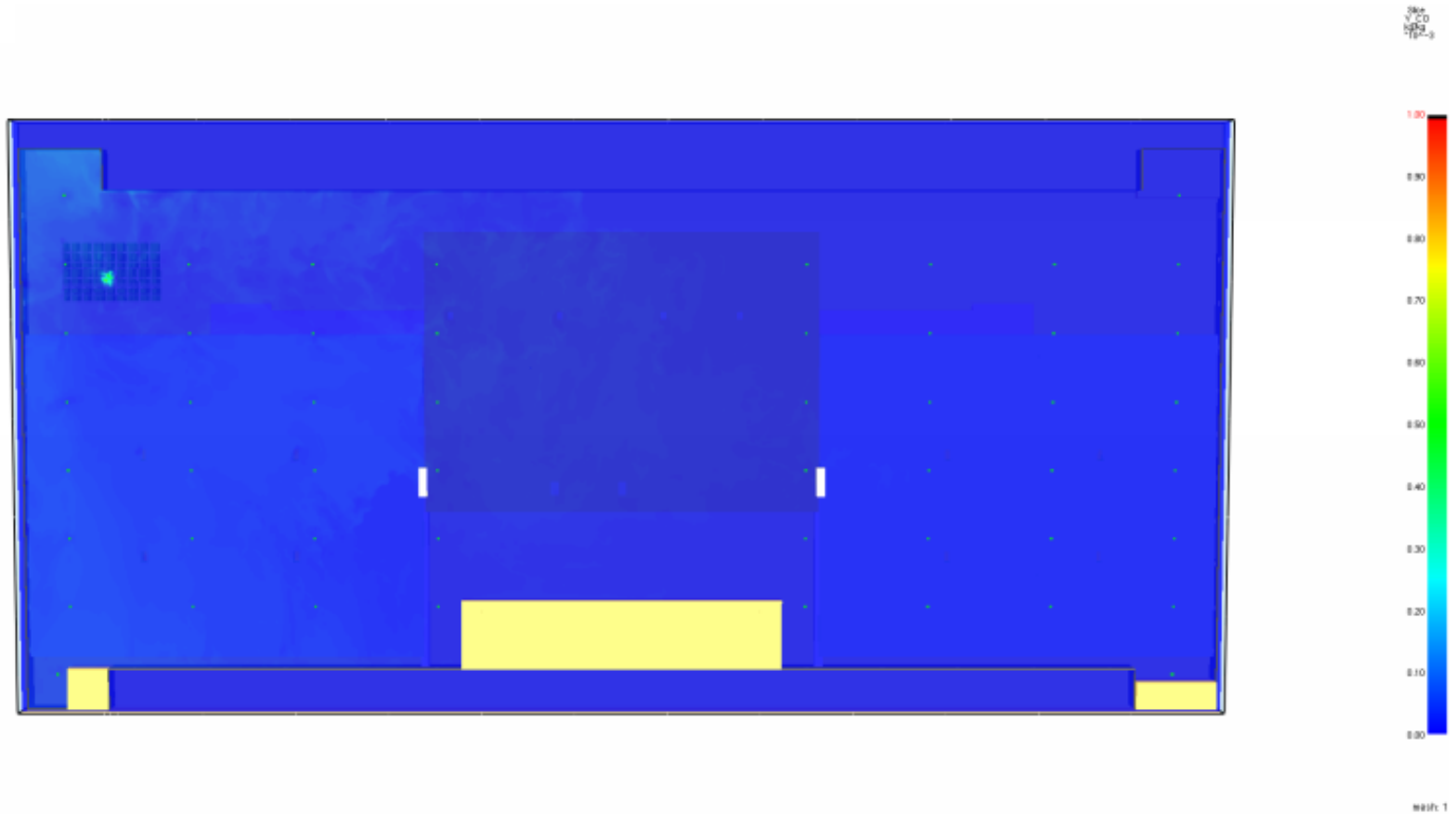
Figure 22: Scenario #1 – CO Concentration at 28 ft after 1,200 seconds
