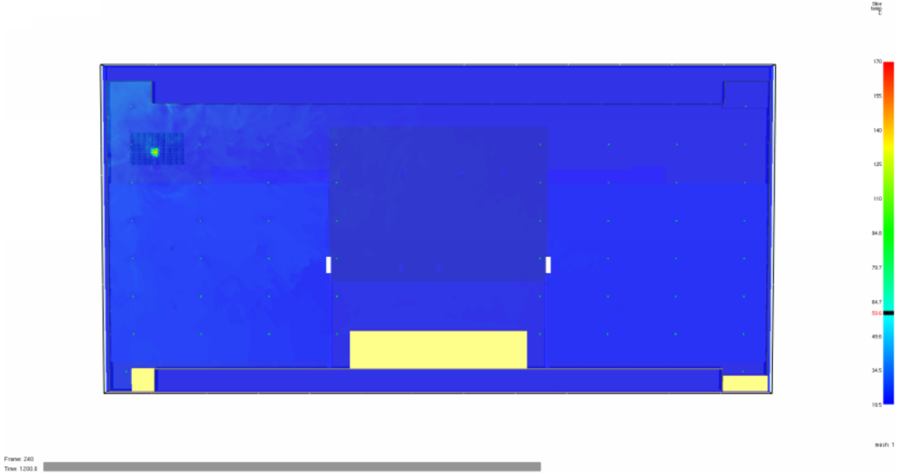
Figure 23: Scenario #1 – Temperature at 28 ft after 1,200 seconds
