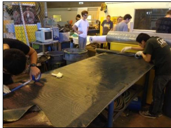
Figure 86. Cutting carbon fiber to size.
