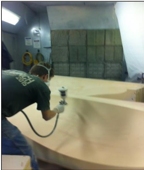
Figure 83. Molds were sprayed with Duratec Sealer and EZ Sand Primer using a paint spray gun.
