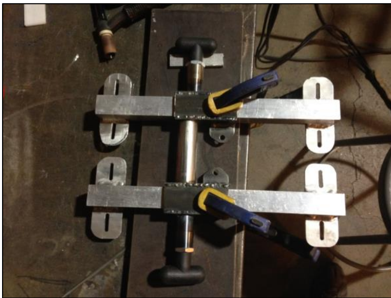
Figure 102. Steel rails and aluminum rails fixtured for welding.
