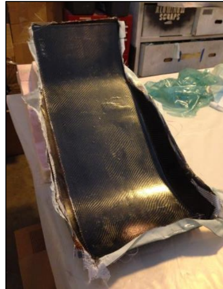
Figure 101. Seat released from the mold with exposed core requiring edge closeouts.
