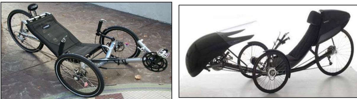
Figure 16. Left: Direct knuckle (Catrike Expedition). Right: Over-seat tiller (AVD Windcheetah).
