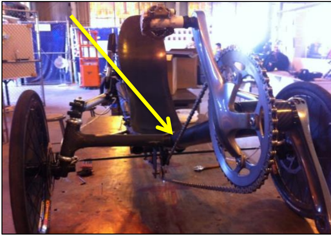
Figure 9. Strut debond and lug cracking that debilitated Aria.
