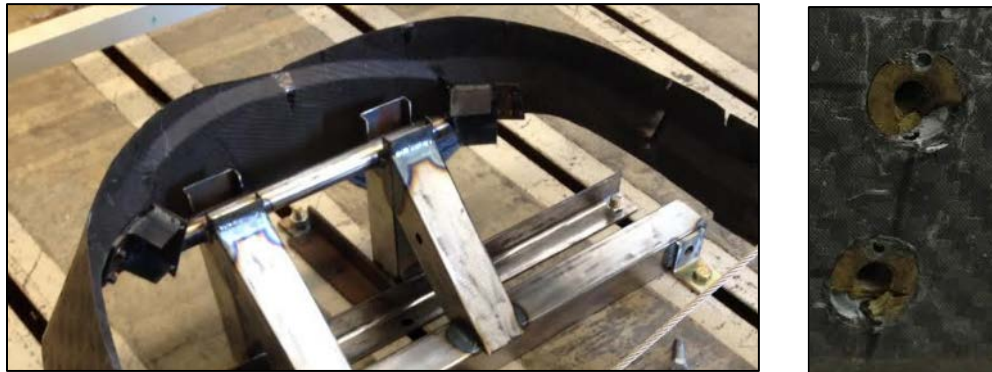
Figure 120. Close up of the boundary conditions (left) and failed potted inserts (right).
