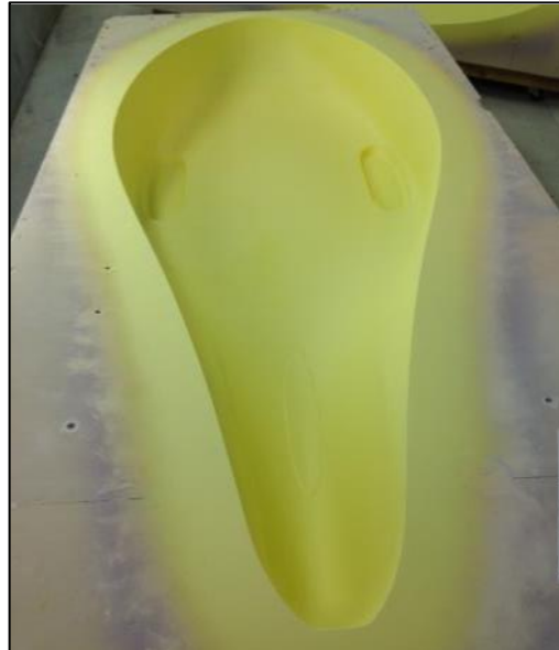
Figure 83. Molds were sprayed with Duratec Sealer and EZ Sand Primer using a paint spray gun.
