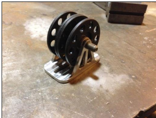
Figure 59. Side-by-side chain routing initial design
