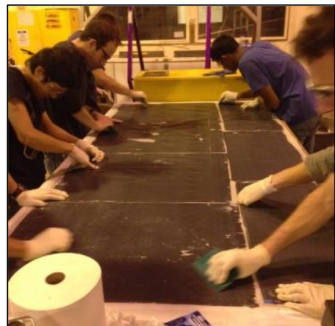
Figure 88. Wetting out carbon fiber.
