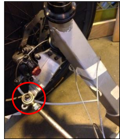
Figure 39. Prototype knuckle with adjustable steering ratios.
