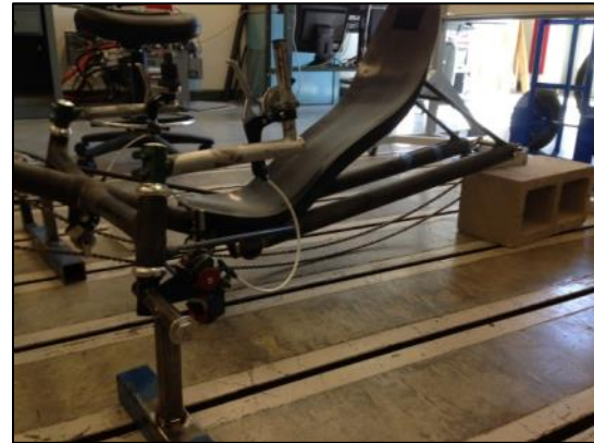
Figure 51. Aria's fixed seat design. This design used spacer pads behind the rider's back to adjust sizes.
