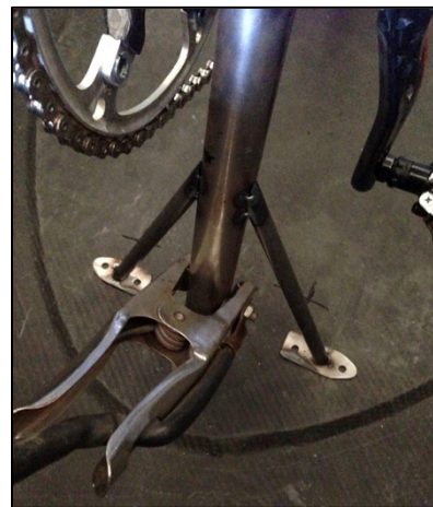
Figure 124. Additional struts welded to BB mount.
