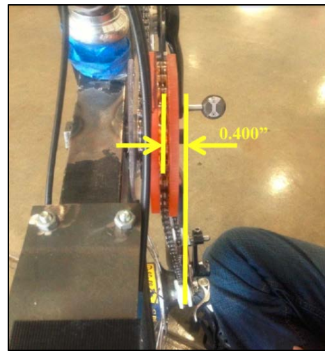
Figure 7. The chain-twist design implemented on Black Stallion. The chain twist caused seizure in the drivetrain, drastically lowering efficiency.
