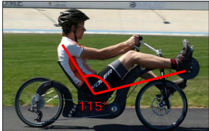
Figure 13. Hip angle is defined as the angle between shoulder, hips, and vehicle bottom bracket.
