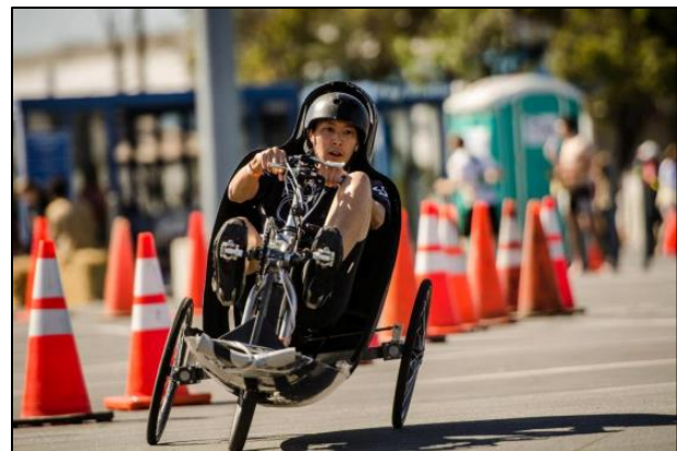
Figure 6. Black Stallion's lean mechanism in action. The nose of the fairing had to be cut off due to a low speed crash from instability at low speeds.
