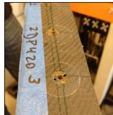
Figure 49. Face sheet failure of potted inserts subjected to tensile loading.
