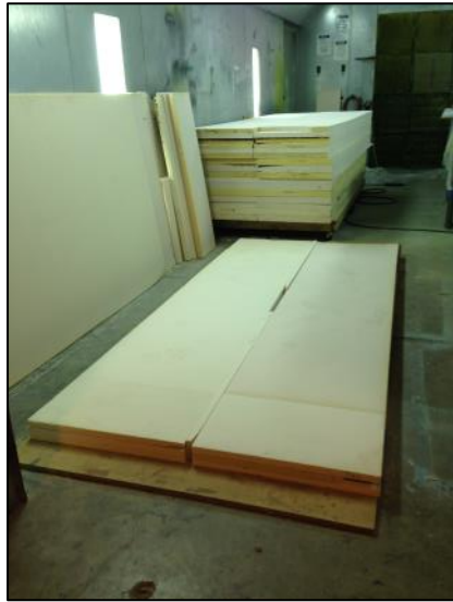
Figure 81. Gluing of foam to create stock for tools. The foam was laid up in blocks of three (left) and guerilla glue was used to adhere the layers. Weight was used to minimize separation between layers of foam while curing.
