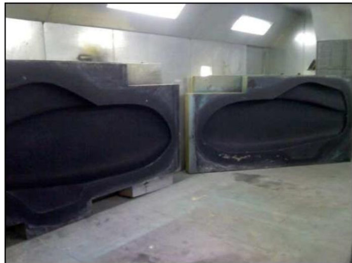
Figure 35. HDU foam molds that the team has traditionally made. The foam is CNC machined and finished with Duratec, a sandable mold sealer.
