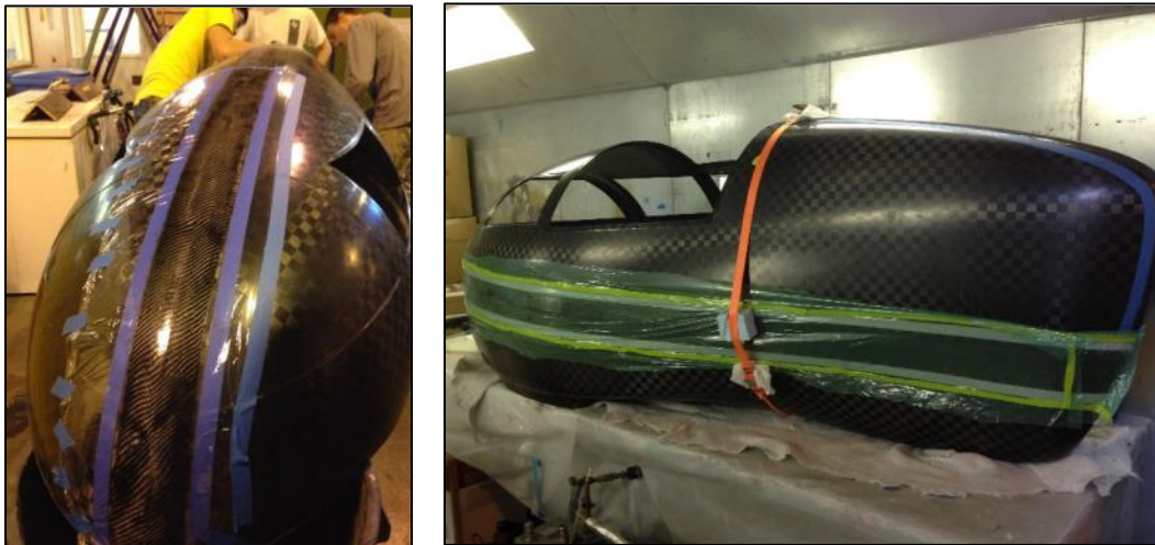
Figure 92. Saran wrap technique for seaming (left) and secondary post-bond inside the fairing with vacuum pump (right).
