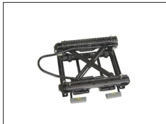
Figure 50. Car seat adjustment mechanism. This would allow for the most effortless seat adjustment, but would require overly complex and heavy mechanisms.
