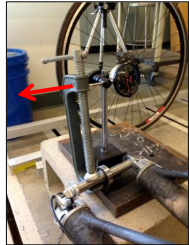
Figure 34. Torsional testing setup with applied force location.
