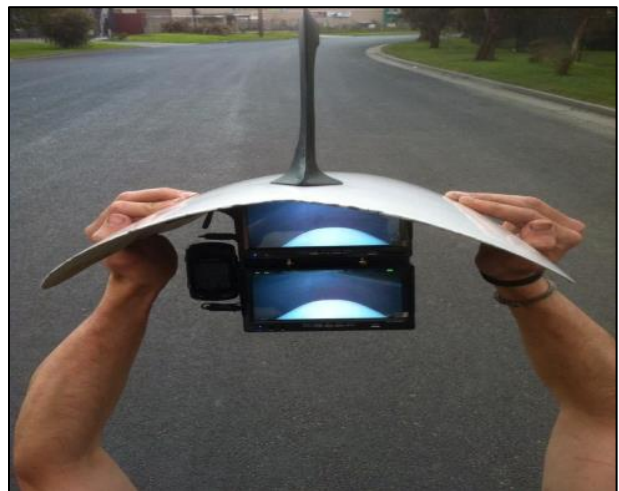
Figure 22. Trisled's All-Overzealous camera configuration. The sting at the top holds two cameras wired independently to the redundant monitors below.
