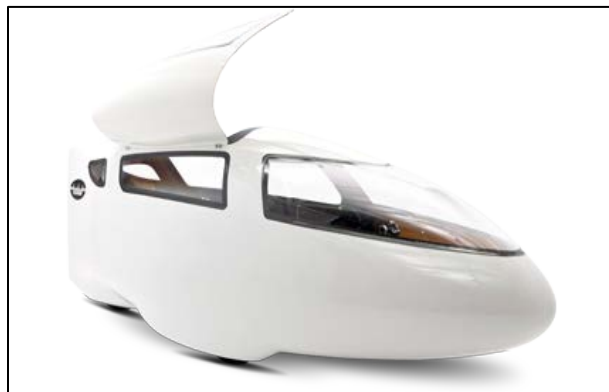
Figure 40. Trisled Aquila with an example of a hinged door. The hinges require special mounts to keep concentricity of the pins on the curved mounting surfaces.
