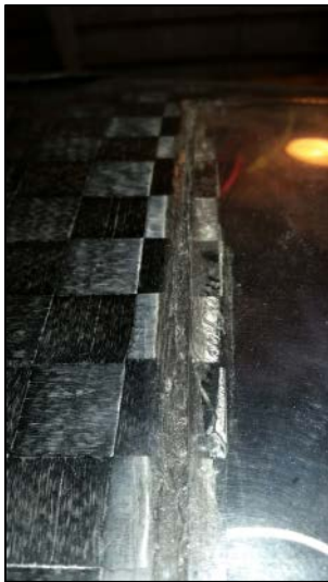
Figure 111. Silicone caulking used to secure the windshield and fill the seams.
