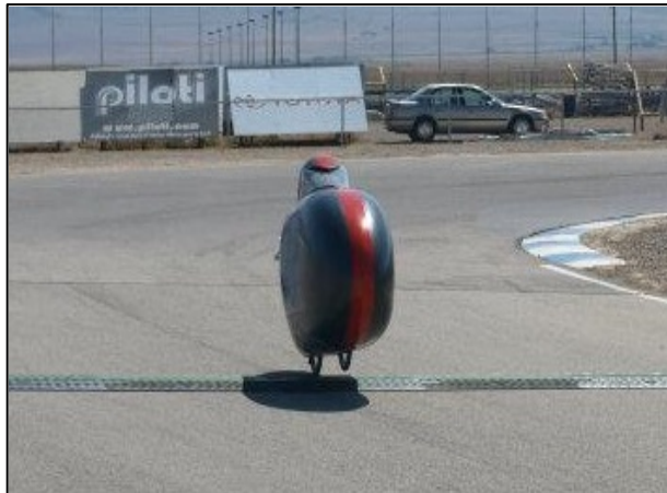
Figure 4. Gemini's high vertical stiffness caused it to launch off speedbumps and caused an uncomfortable ride quality.
