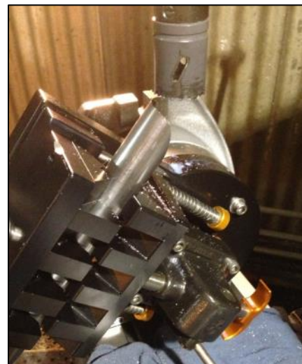
Figure 97. Cutting knuckle mount on tube miter fixture.
