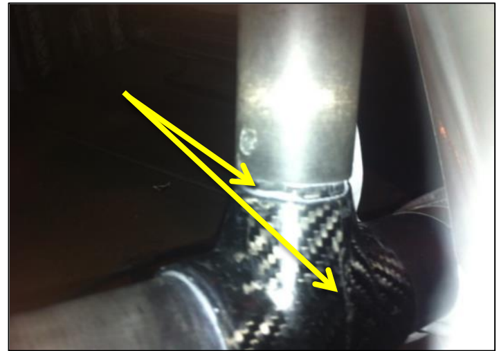
Figure 9. Strut debond and lug cracking that debilitated Aria.
