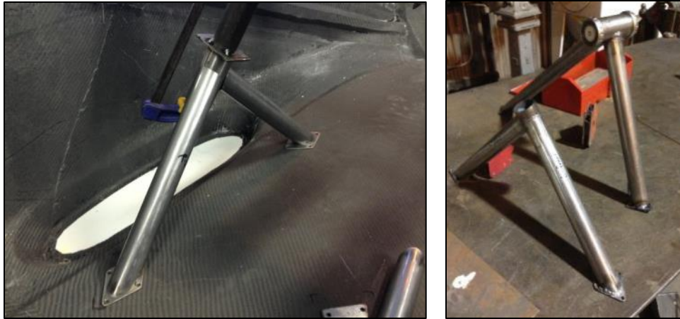
Figure 98. Knuckle mount alignment (left). Full welded knuckle mount and bottom bracket mount (right).
