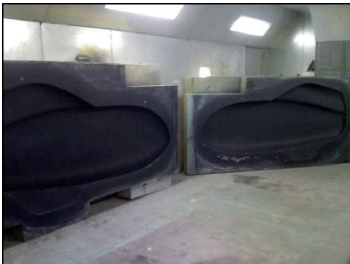
Figure 76. Traditional Cal Poly HPV left / right half molds.
