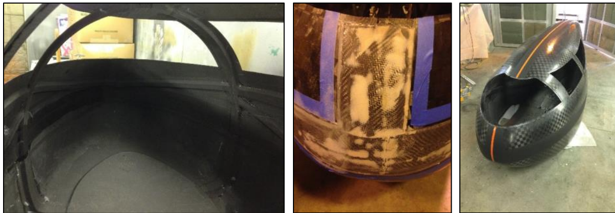
Figure 93. Completed inner seams (left). Outer seam patching and sanding (center). Completed seam with paint (right).
