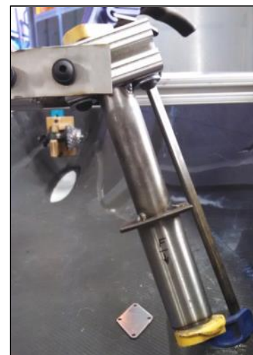
Figure 95. Left axial headtube extension, with headtube clamped in place.
