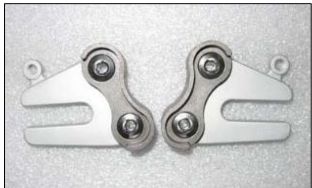
Figure 73. Rear dropouts, as purchased. The lighter colored aluminum pieces were replaced with custom parts with altered slot dimensions and orientations.
