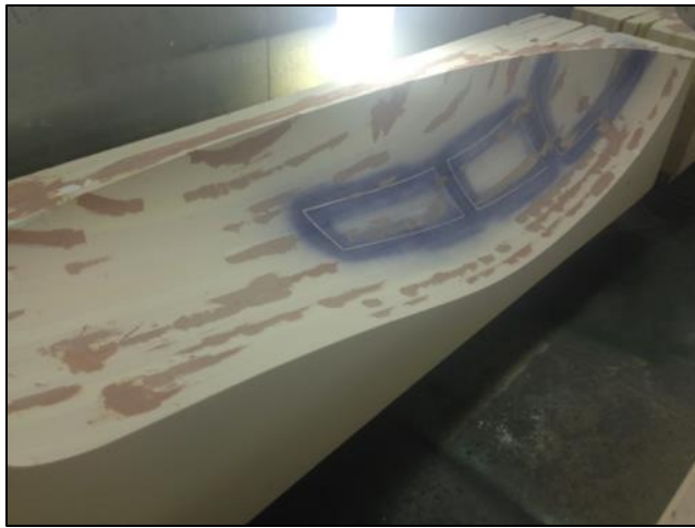
Figure 84. Initial foam sanding and Bondo® application before spraying Duratec primer.
