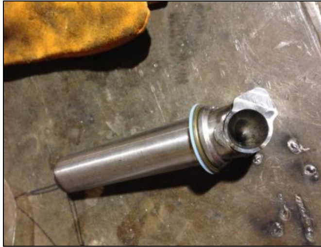
Figure 114. Welded bore and steerer.
