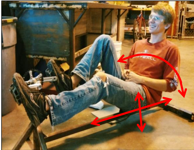
Figure 15. The rider position jig used to verify seat locations for each rider. The bottom bracket location is fixed, and arrows show the available seat adjustments.
