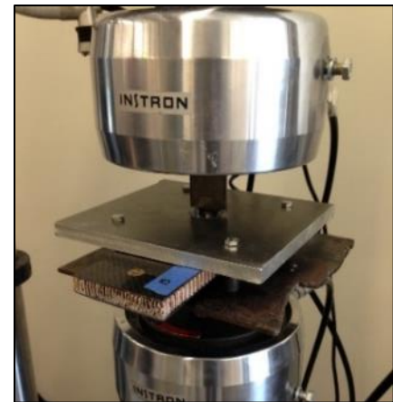
Figure 48. Potted insert testing setup.
