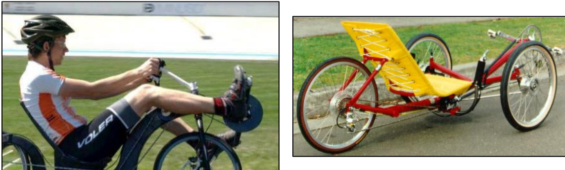
Figure 17. Left: Over-seat push/pull (Gemini, 2012). Right: Under-seat rotation (Greenspeed GTS).
