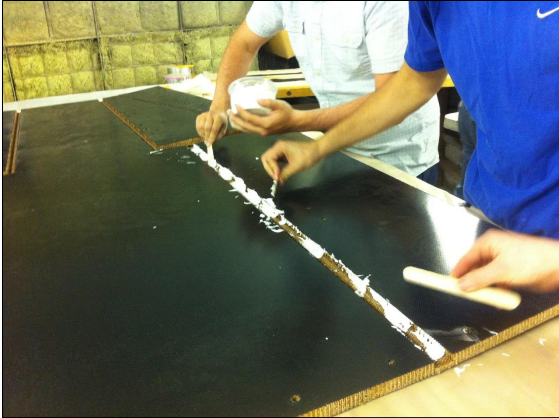
Figure 5.5: Application of resin and microballoons to groove in panel.
