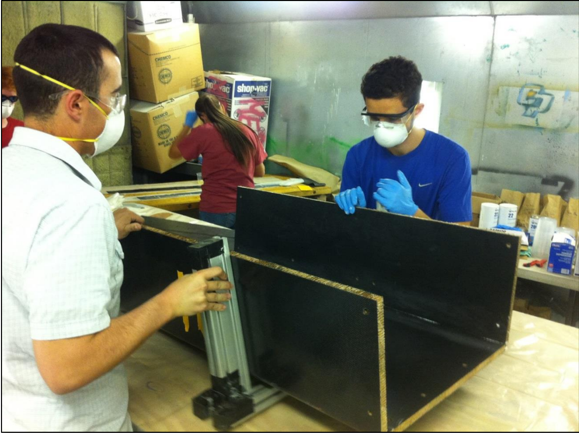
Figure 5.8: Locating panel in jig.
