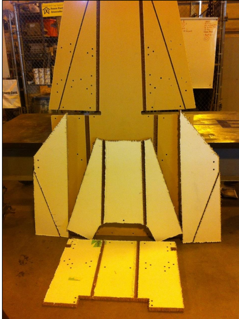
Figure 5.2: Fiberglass panels after CNC routing.
