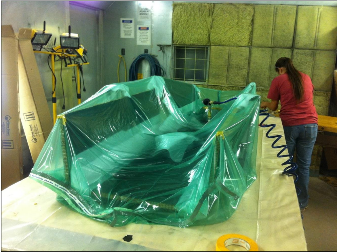
Figure 5.12: Vacuum bag sealed around panel.
