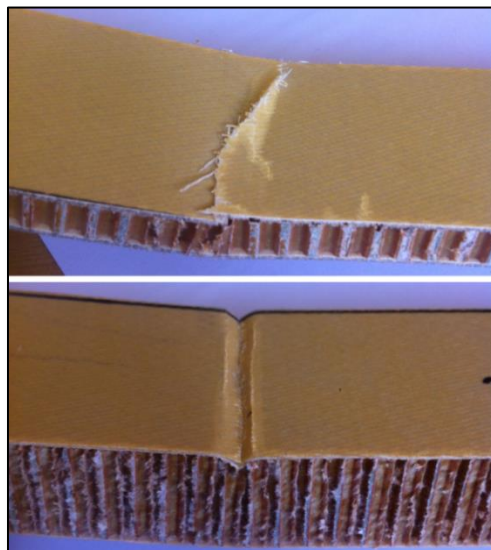
Figure 3.34: Thinner (Top) and Thicker (Bottom) Panel Failure Modes For Long Beam Test
