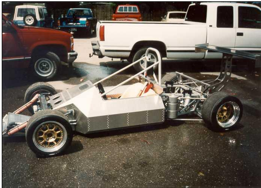
Figure 2.4: Aluminum monocoque formula chassis.
