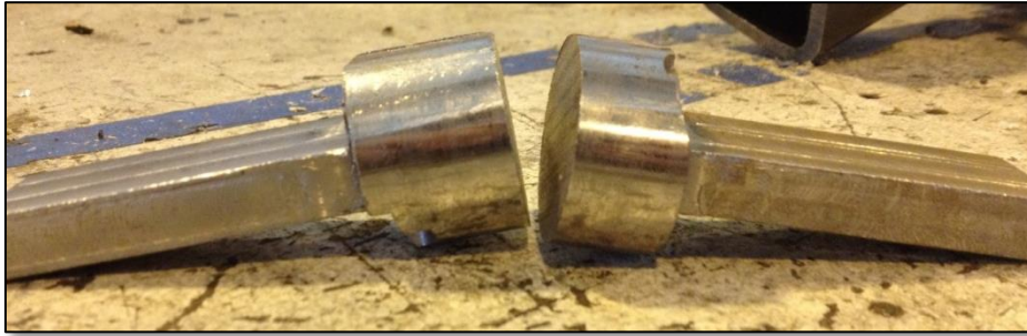
Figure 3.27: Core Crushing Fixtures
