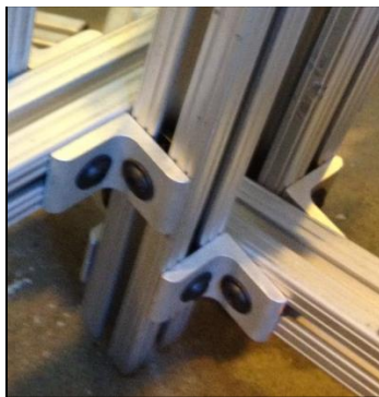
Figure 3.12: Double Bracket System to Allow Rotation of Vertical Mockup Components
