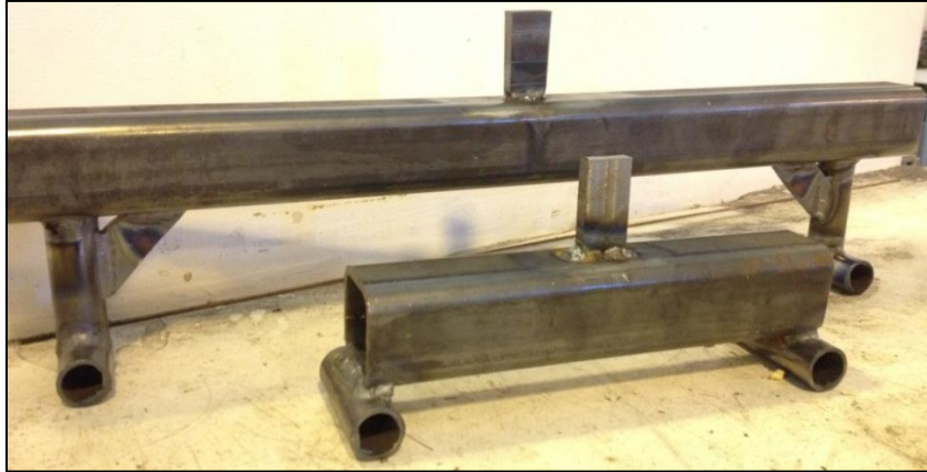
Figure 3.24: Long Beam Fixtures
