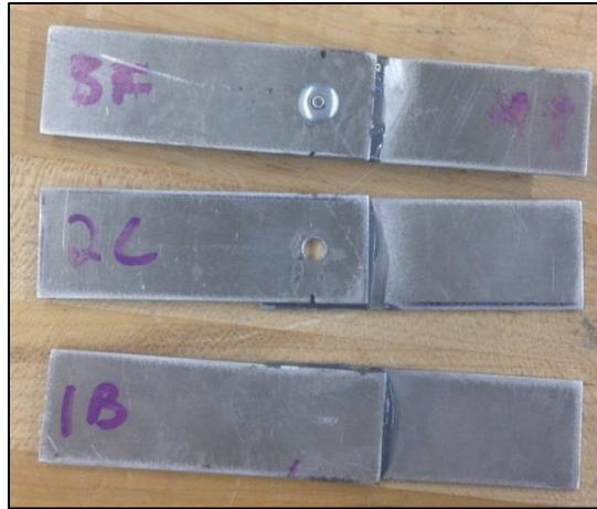
Figure 3.5: Samples from the Three Adhesive Testing Groups.
