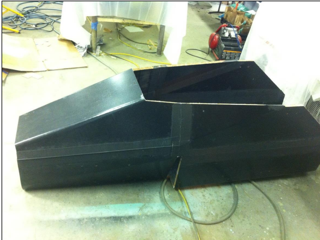
Figure 5.15: Carbon chassis with completed bend reinforcements and lap joints.
