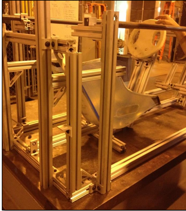
Figure 3.11: View of Cockpit Mockup Showing Seat Mounting, Top Tube Mounting, and Steering Wheel
