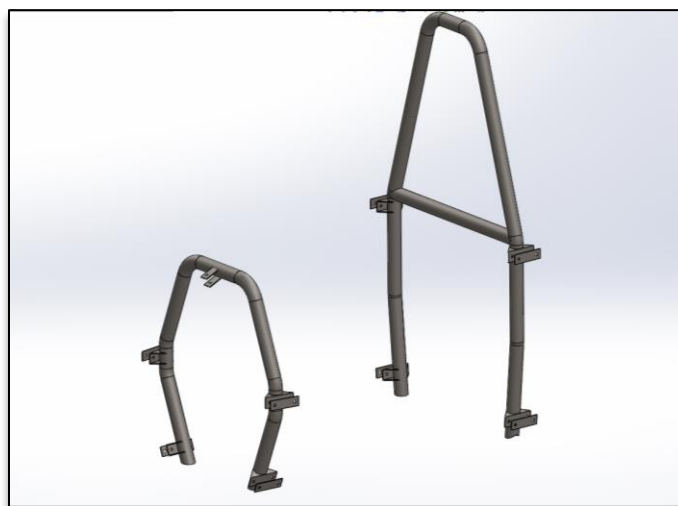
Figure 4.6: Roll Hoops and Mounting
