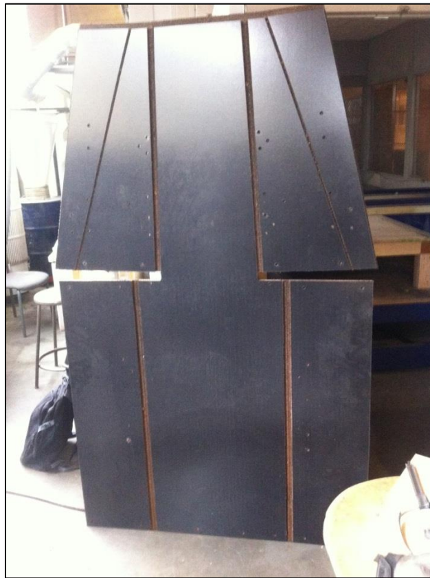
Figure 5.4: Finished carbon panel after removal from the router.
