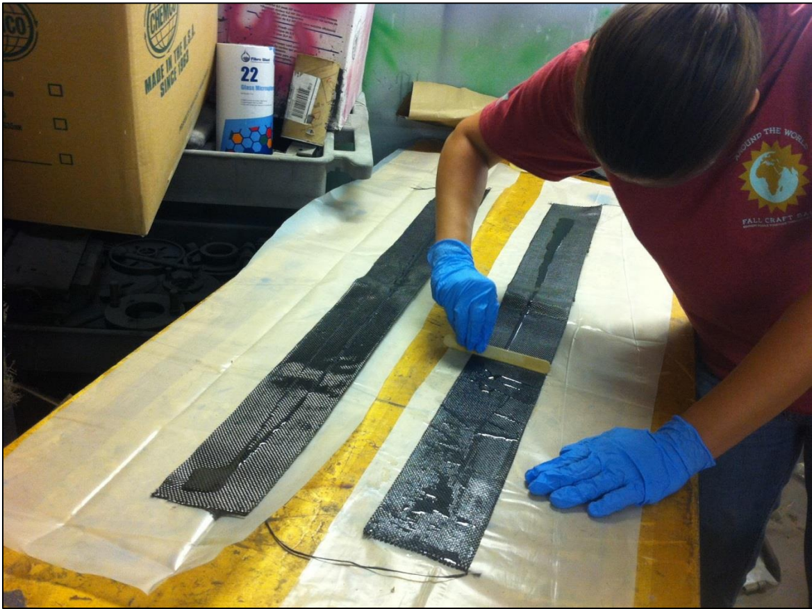
Figure 5.6: Resin being spread onto carbon tape to wet entire surface.
