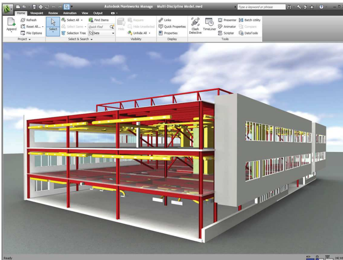
EXAMPLE NAVISWORKS FROM AUTODESK'S WEBSITE ILLUSTRATING HOW ONE CAN COMBINE STRUCTURAL, ARCHITECTURAL, MEP, AND OTHER SYSTEMS IN NAVISWORKS
