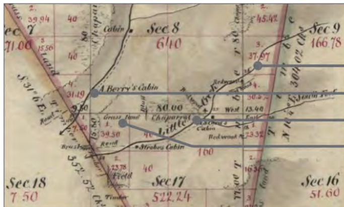
Figure 6: Traverse Line Run from Redmond Post A.P.5 to Large White Post A.P.6. U.S. Coast Survey. 1868 General Land Office Records (GLO) Rancho Agua Puerca y Las Trancas Plat Map. The top image provides a basic survey of the land grant boundaries. While this map is sparse in features, it conveys surveyor notations of what line was used to determine the distance of the Rancho and the boundary of its neighbor Rancho San Vicente. The bottom image provides a more detailed version of the area. United States Department of Interior, Bureau of Land Management, General Land Office Records, DM ID 380771, Lauren Upson (Surveyor General), 1868, http://www.glorerecords.blm.gov/details/survey/default.aspx?dm_id=380772&sid=h3jklvyg.mci&surveyDetailsTabIndex=1#surveyDetailsTabIndex=1 .
