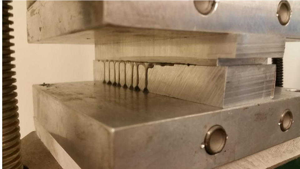
Figure 3.14. Resin leaking out of 3-point bend specimen mold upon pressure application.
