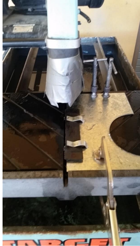
Figure 2.23. Flash-trimming jig clamped to the wet diamond saw with tensile specimen.
