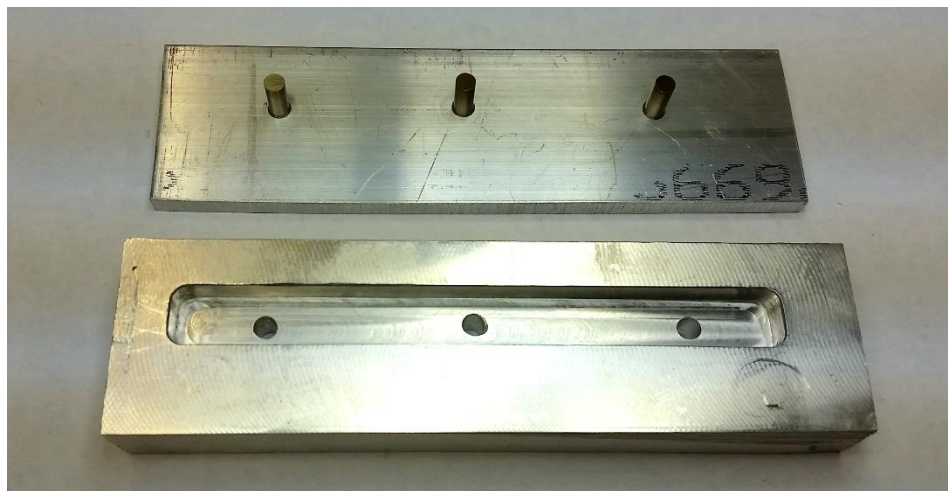
Figure 3.8. Finished mold cavity with ejector pin plate.
