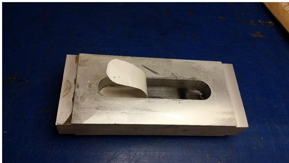
Figure 4.7. First face sheet placed into pin-loaded tensile specimen mold.
