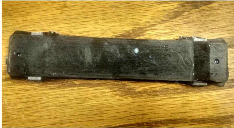
Figure 2.18. 14-ply P35/Z03 part with holes from machining ejector pins.
