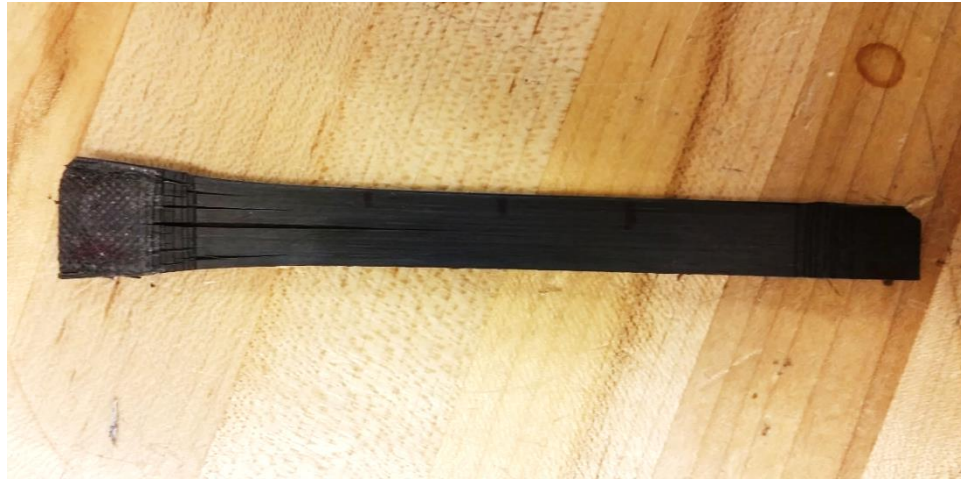
Figure 2.29. 15-ply P35/Z03 tab "brooming" failure from clamping in Instron grips.
