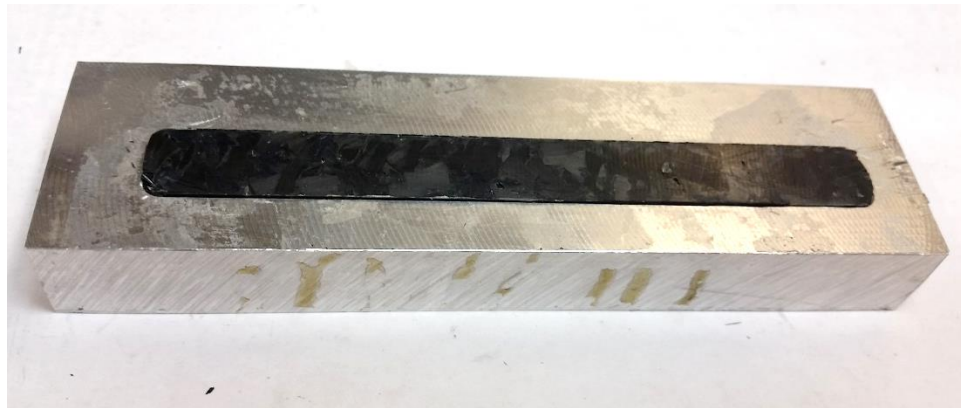
Figure 3.15. Chopped fiber 3-point bend specimen ejected from mold cavity.
