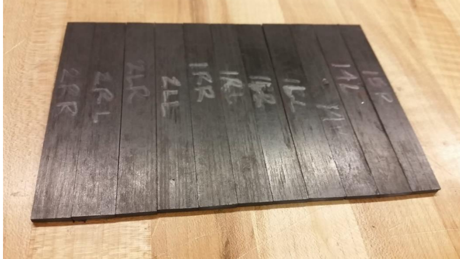
Figure 2.30. Tensile specimens trimmed into 3-point bend specimens.
