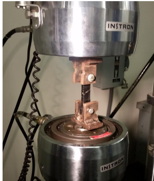
Figure 4.10. Test setup used to evaluate pin-loaded tensile specimens.
