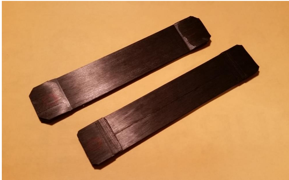
Figure 2.15. First compression molded parts: 10-ply P35/Z03 tensile specimens with tabs.
