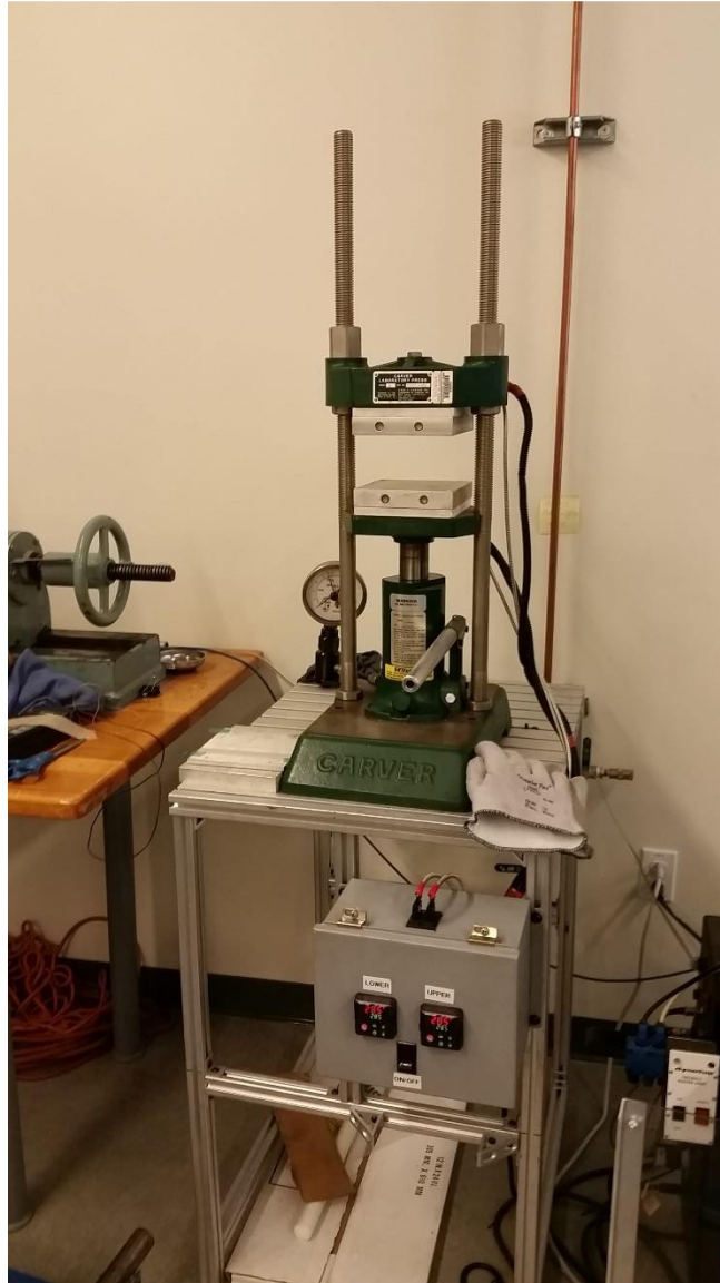
Figure 2.1. Carver press setup used for compression molding.
