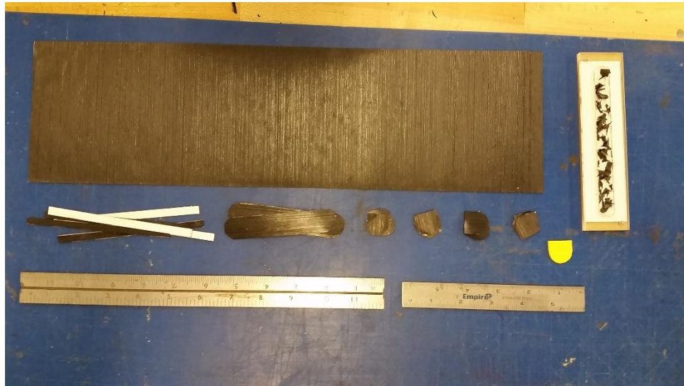
Figure 4.6. Required material for one pin-loaded tensile specimen.
