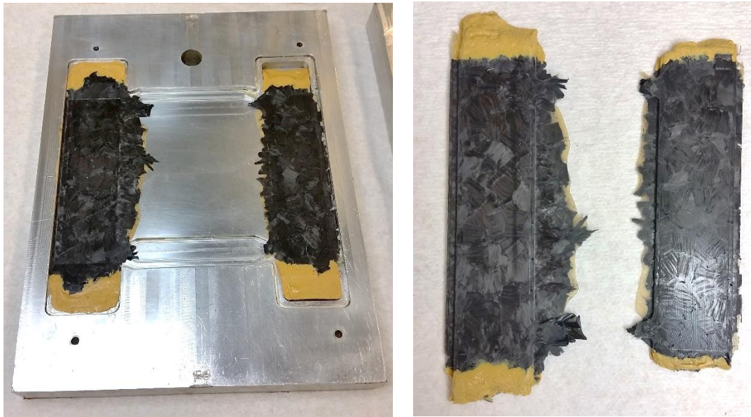
Figure 3.5. First compression molded chopped fiber parts.
