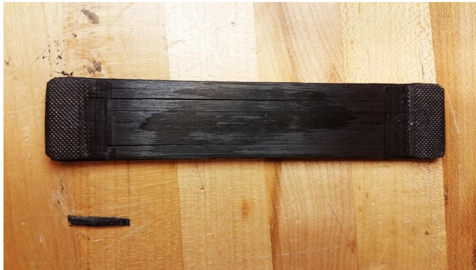
Figure 2.28. "Brooming" failure mode experienced by a 10-ply P35/Z03 tensile specimen.
