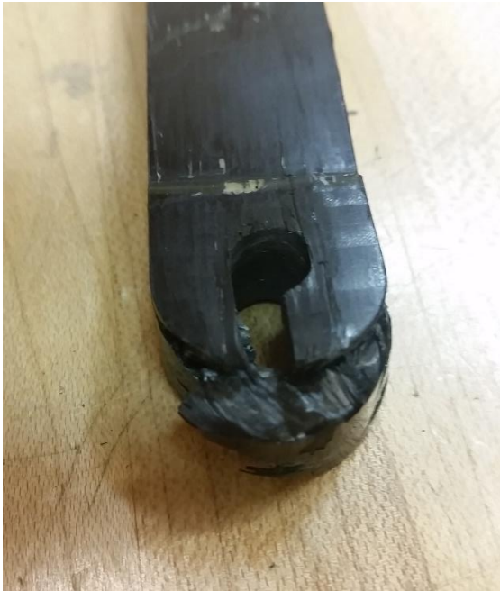
Figure 4.11. Catastrophic cleavage and shear-out failure mode.
