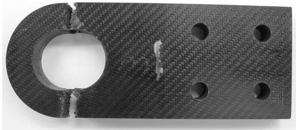
Figure 4.1. Example of a composite lug which has failed in net-tension [50].
