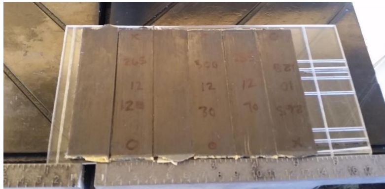
Figure 2.44. M46J/TC250 3-point bend specimens prepared for ripping.
