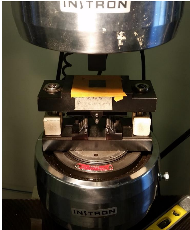
Figure 2.34. 3-point bend apparatus set up on Instron load frame.
