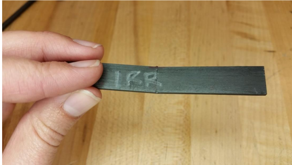
Figure 2.36. Microbuckling failure mode of 3-point bend specimens.
