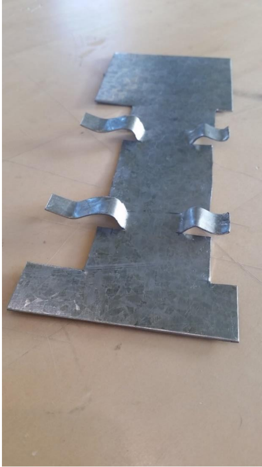
Figure 2.22. Finished flash-trimming and specimen-ripping jig.
