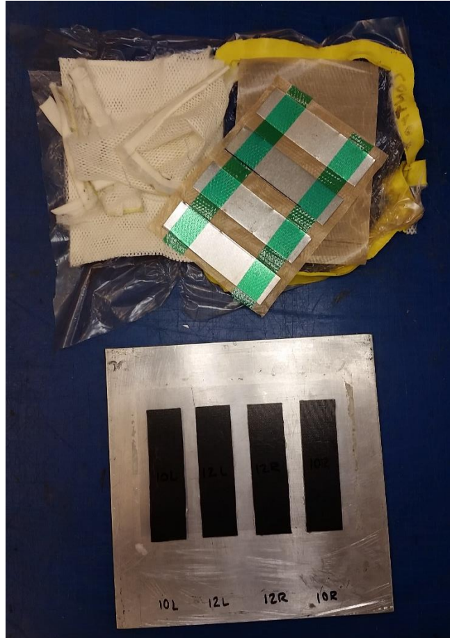
Figure 2.51. Fully cured autoclave specimens and used bagging material.
