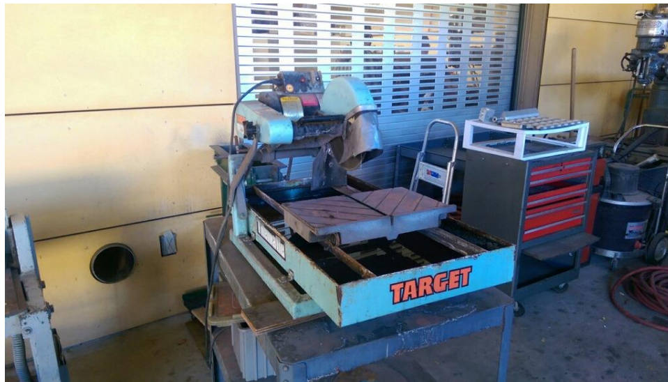
Figure 2.21. Wet diamond saw used to trim and rip specimens.
