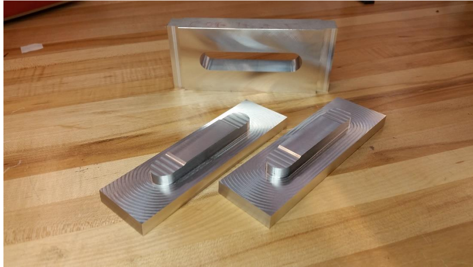
Figure 4.5. Finished 3-part lug mold.
