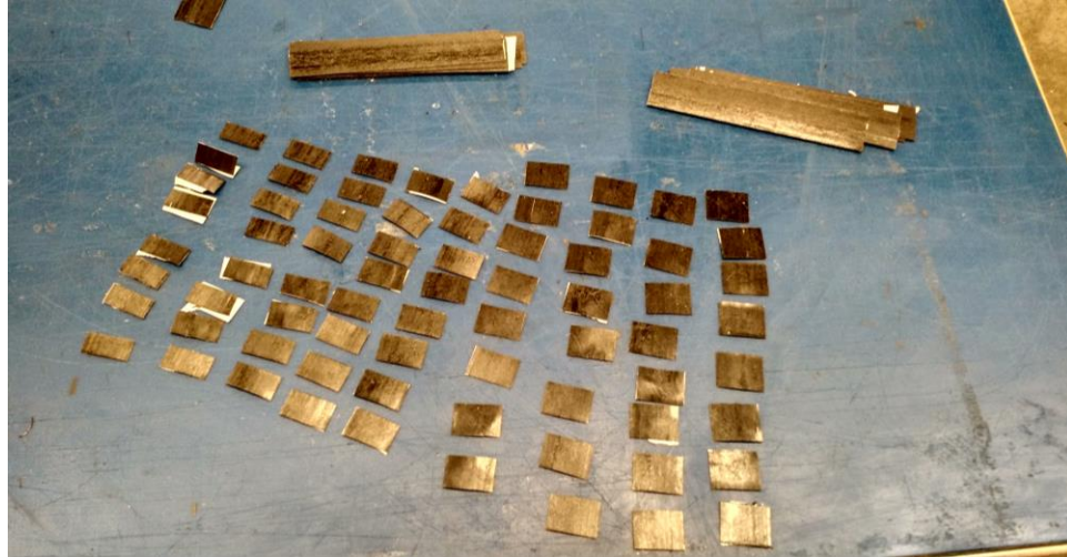
Figure 2.10. Plies for two tensile specimens and tabs.
