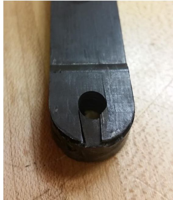
Figure 4.12. Bearing failure mode caused by quasi-static loading.
