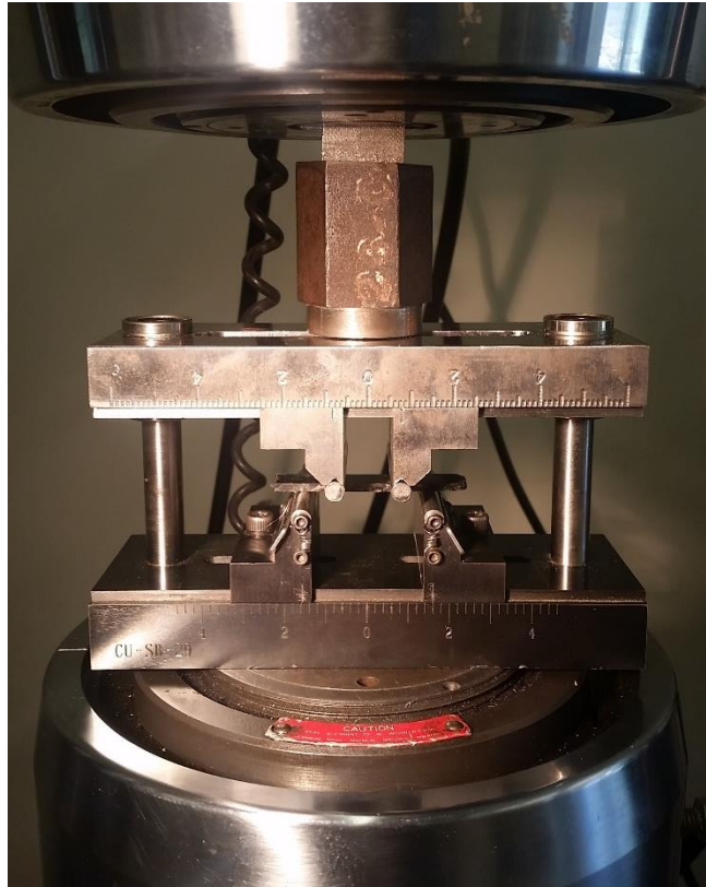
Figure 3.18. 4-point bend apparatus set up in Instron load frame.
