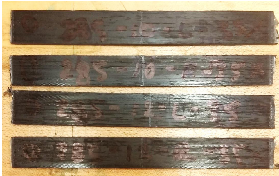
Figure 2.45. Representative tested M46J/TC250 3-point bend specimens.
