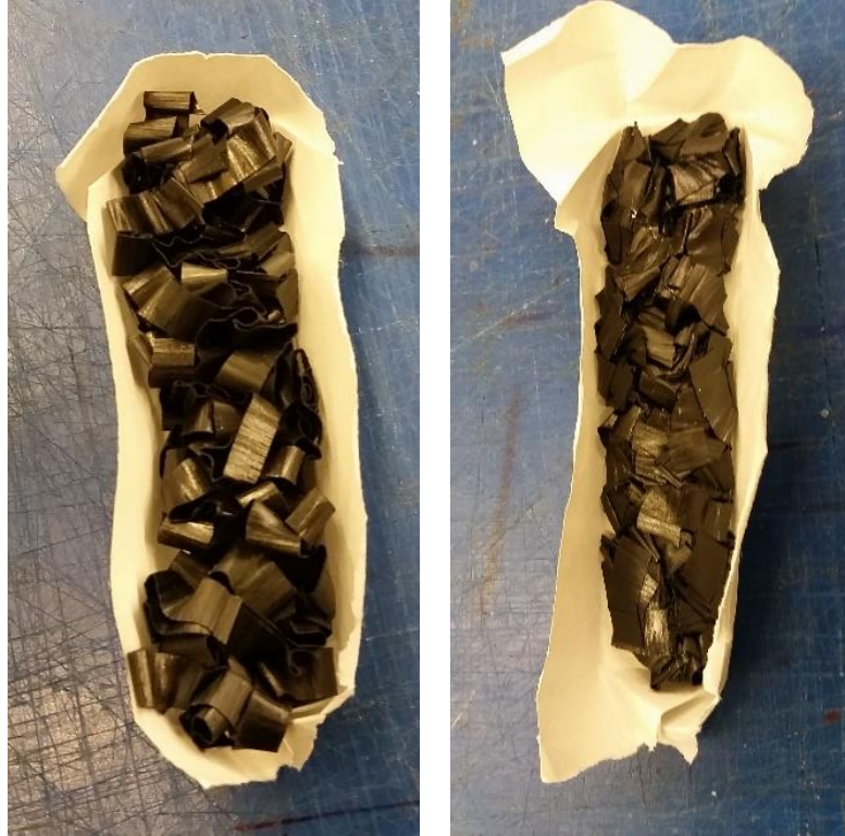
Figure 3.6. Preformed 0.25 in strips formed by Method #3.
