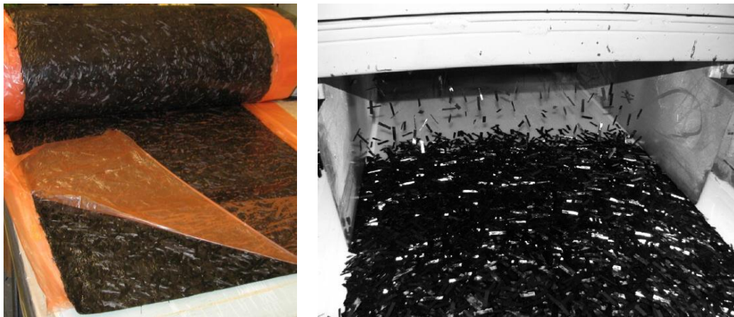
Figure 1.2. SMC (left) and BMC (right) material forms used for compression molding [6].
