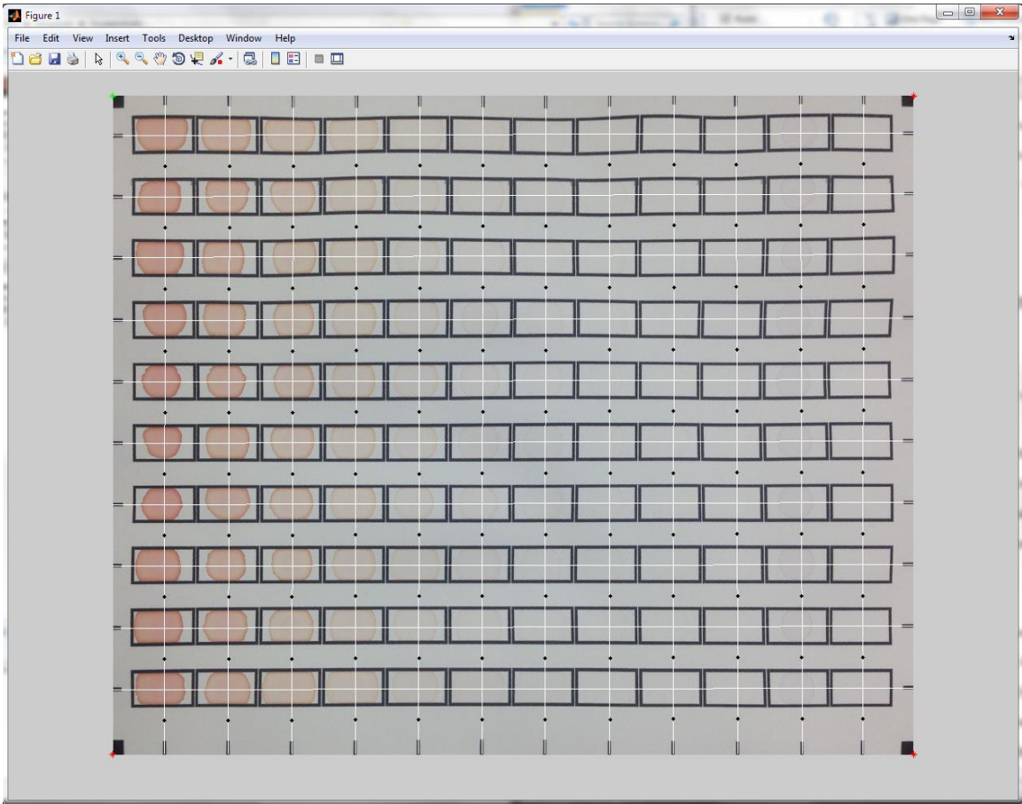
Figure 21. Partially processed image displayed in MATLAB, with column and row centerlines (white) and reference locations (black diamonds) superimposed on it. Intersections of the white lines are sample data collection locations.
