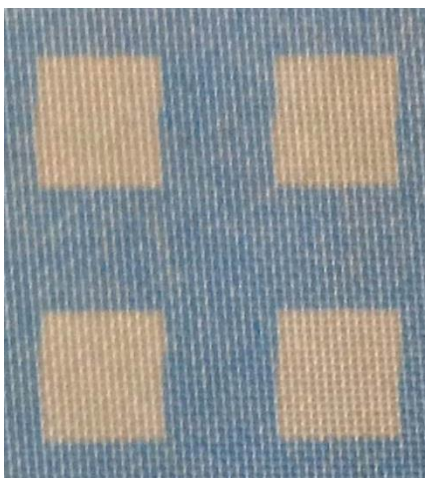
Figure 26. Close-up photograph of electrode negative used for screen printing.
