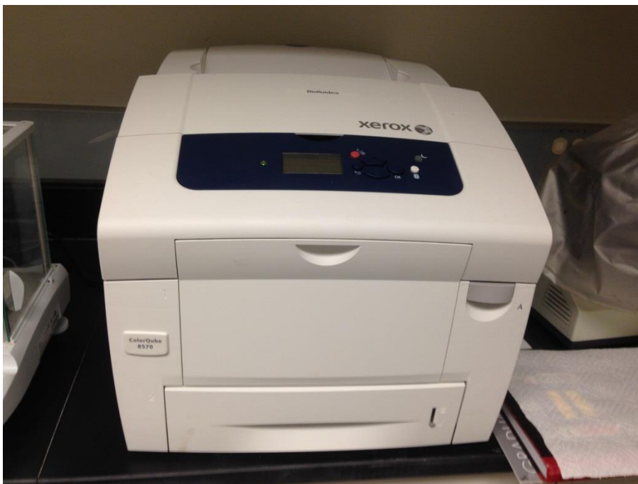
Figure 7. Xerox ColorQube 8570 solid ink printer used for printing hydrophobic wax barriers on nitrocellulose.
