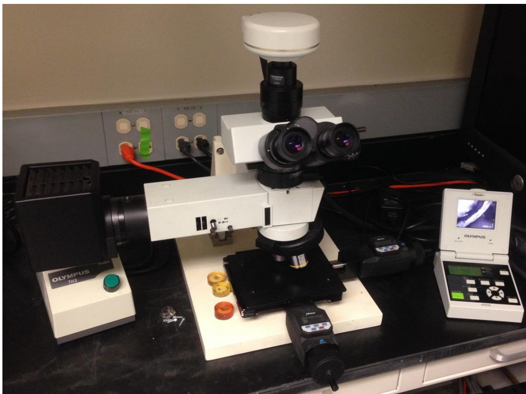
Figure 23. Olympus microscope with camera unit used for capturing images of samples on NC.
