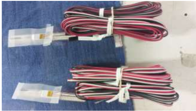
Figure 30: Two bipod rods during the strain gauges bonding process.
