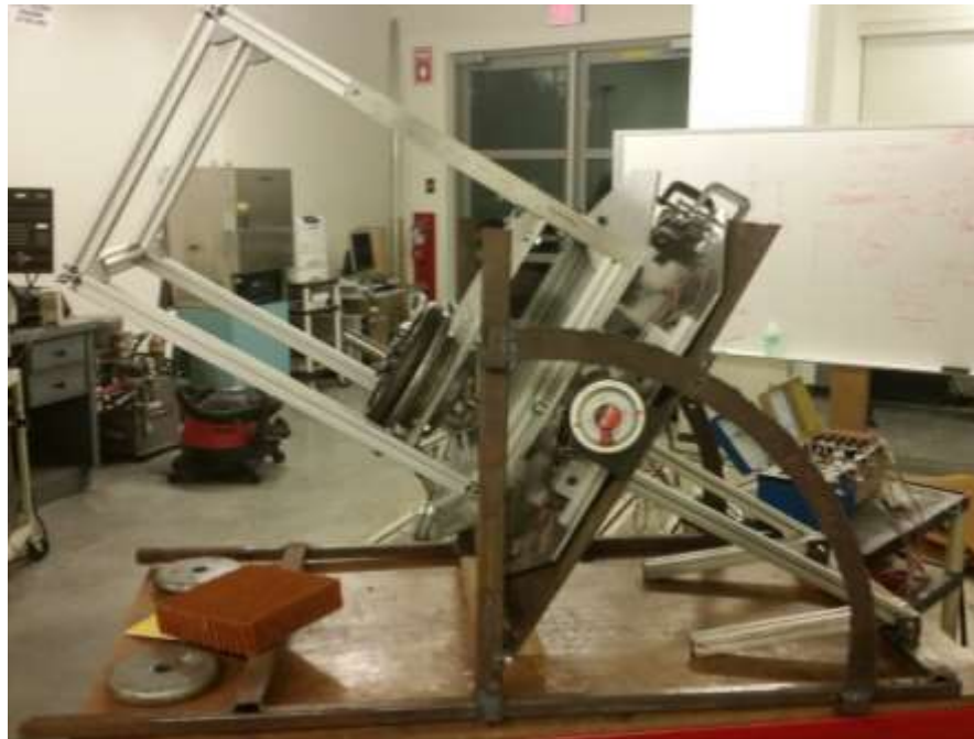
Figure 46: Test at \alpha = 60^0 with 35 lbs payload (nominal) and the self-height set to 5.5in.
