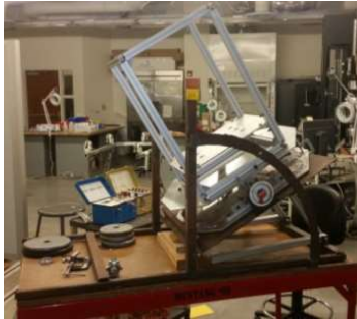
Figure 45: No load Test with \alpha = 30^\circ tilt.
