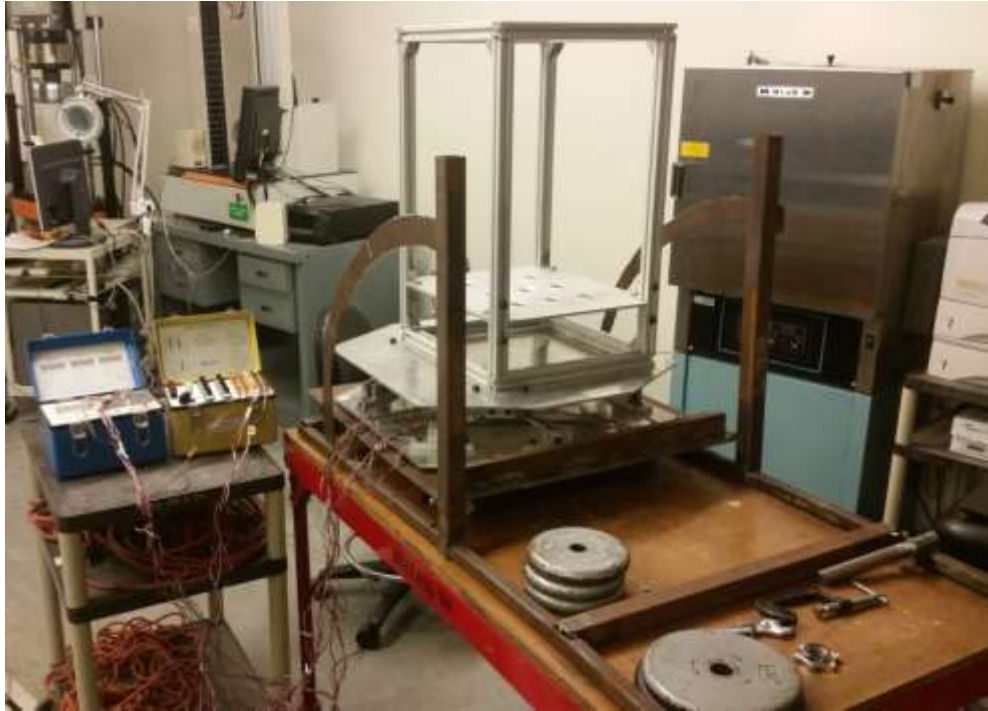
Figure 43: Test set up using the P3 strain indicator (Blue box) and the Switch Terminal (Yellow box) as a DAQ.
