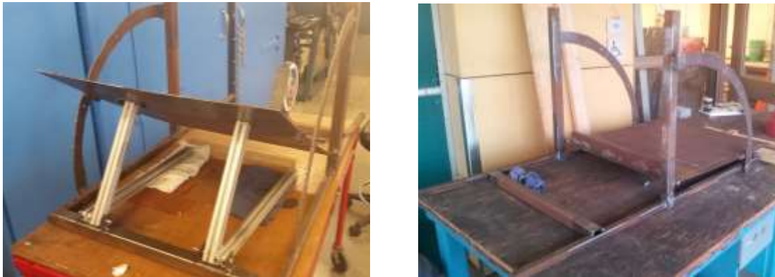
Figure 33: (Left) Rear view of the tilt table at 30°. (Right) Front view of the tilt table at 0°.
