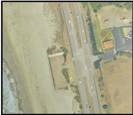
Location: PM 32.5 Size: ~10 spaces Visitor Amenities: None Ingress/egress: 1 60' left-turn lane, 8 foot shoulders Planned Improvements: - TBD
