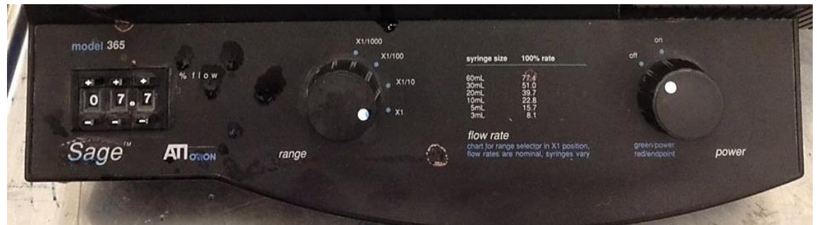
Figure 18: Mechanical Pump Control System
