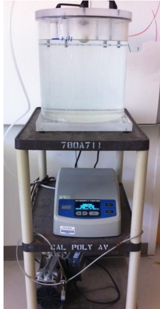
Figure 19: Test-A-Pack Machine for Hermeticity Testing
