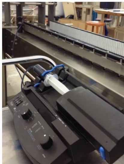
Figure 6: Mechanical Syringe Pump Setup
