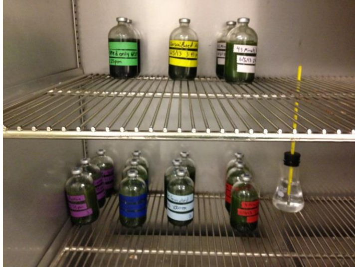
Figure 15. Assembled triplicate digesters sitting in the 35\pm 2^{\circ}\text{C} incubator. All of the digesters pictured are 160-mL serum bottles, but in some experiments, custom 2-L digesters with septa were used to have enough digestate for experiments on aerobic degradation Chang (2014) and allelopathy of regrowth Boggess (2014).
