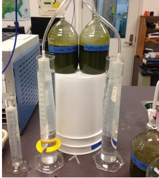
Figure 17. Setup for measuring biogas yields of the 2-L digesters. Graduated cylinders (250 mL) were adapted with silicone and ¼ inch barbed fittings and inverted in 1000-mL graduated cylinders to measure the volumetric gas production.
