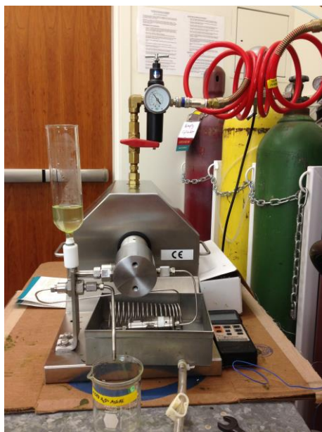
Figure 10. Front view of the Microfluidics pneumatic M-110L cell homogenizer. The unit is pneumatically powered and has a large piston that compressed air up to 20,000 psi. Untreated samples were loaded into the glass hopper on the left, and treated samples exited the downspout in the front, and were collected in a beaker.
