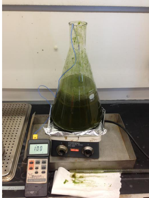
Figure 13. A 4-L Erlenmeyer flask was filled with 1200 mL of tube settler harvested algae and stirred with 5-cm long magnetic stir bar. A combination hot plate stirrer was used to heat the algae to 100°C and hold it constant for a period of 30 minutes.
