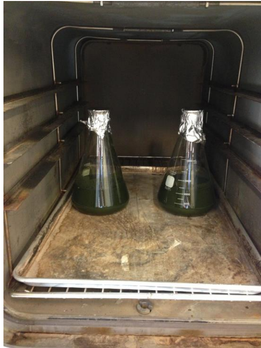
Figure 12. Flask spacing was approximately 8 cm at their bases. Considerably more biomass could be treated using the autoclave.
