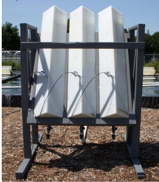
Figure 7. Each pond was connected to a 123 L tube settler packed with nine 3” PVC tubes. The apparatus is positioned at a 60° angle of repose. The influent lines can be seen entering the vessel approximately 1/3 from the bottom. Image source: (Ripley, 2013).
