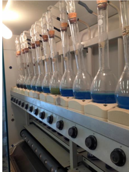
Figure 19. The distillation step of TKN analyses. Distillate (250 mL) was collected in Erlenmeyer flasks and manually titrated using 0.02 N H 2 SO 4 .
