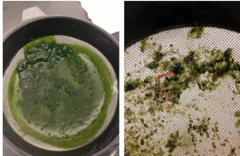
Figure 9. A metal 1-mm screen was used to remove particulates that were clogging the 100- \mu\text{m} Microfluidics interaction chamber. Objects that were removed mostly consisted of ostracods and bloodworms, as seen in the image on the right. Each square in the grid is ~1 mm in size.
