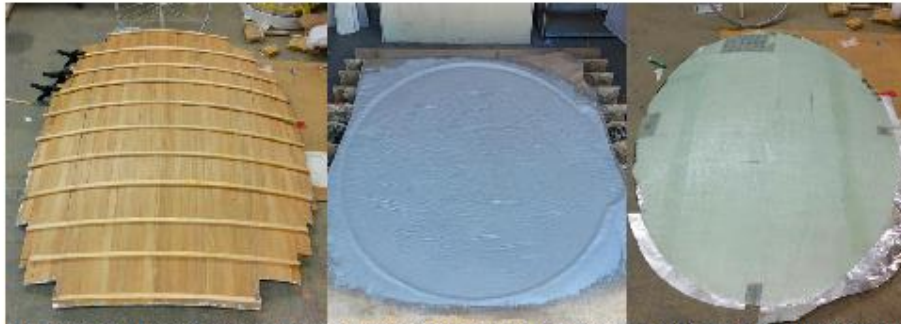
Figure 12 Three possible construction techniques for the secondary parabolic mirror: (left) curved wood slats, (center) concrete latex and burlap composite, and (right) fiberglass.
