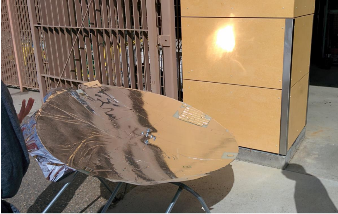
Figure 5.3: Fiberglass reflector prototype with various reflective surface materials
