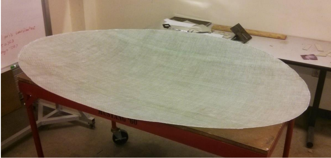
Figure 5.2: First fiberglass prototype before application of reflective Mylar coating
