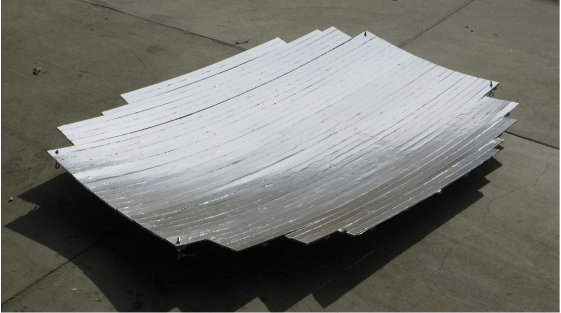
Figure 5.7: The finished wooden reflector prototype with reflective aluminum coated Mylar
