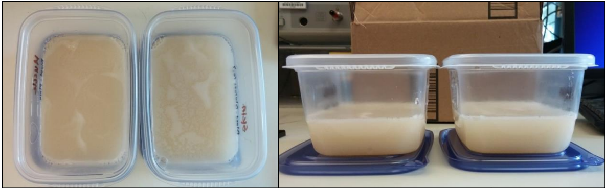
Figure 59: Top view and side view of the two fabricated blood phantoms. One phantom contained no added glucose (left) while the other contained 5 grams of added glucose (right).
