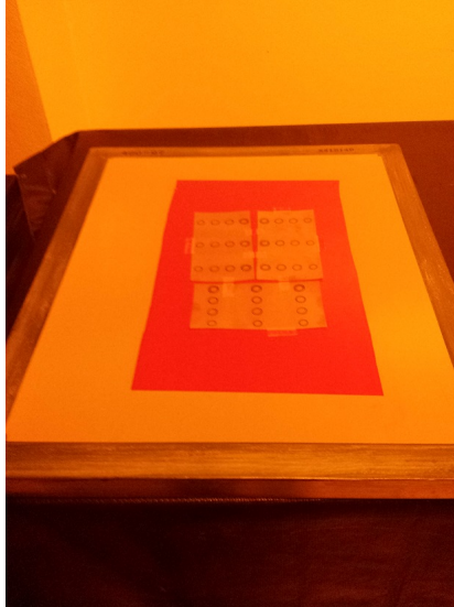
Figure 3.23: Mask Laid On Top of Emulsion
