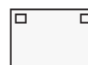
Bare die CBC005 suitable for wirebonding. Dimensions: 1.7mm x 2.25mm x 0.175mm. [Not to scale.]
