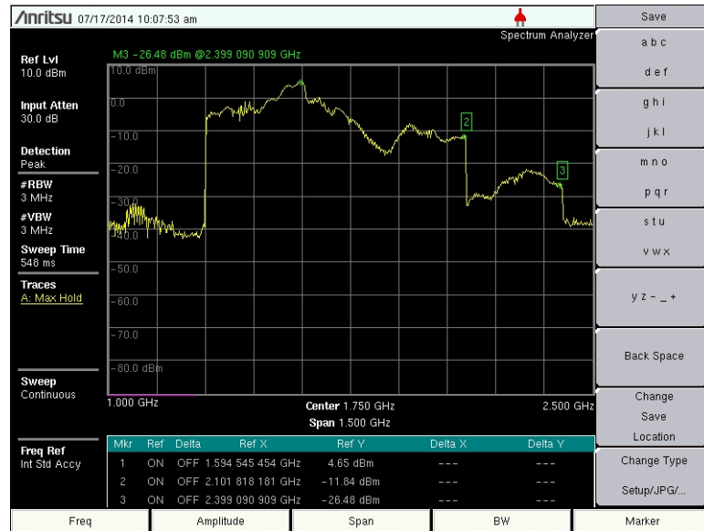
Figure 3.90: Frequency Response of Common Source Amplifier
