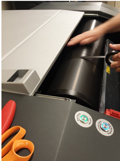
Figure 3.20: Feeding Carbon Sheet into Esko CDI
