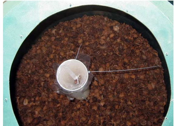
Figure 3.12: Walnut shell packed-bed. Shown before digester operation. Note the slotted PVC pipe at center, which housed the geonet wattle.
