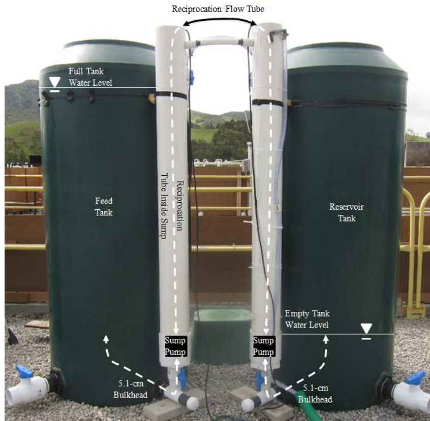
Figure 3.5: Reciprocated flow between tanks. One tank was full while the other remained empty. The water levels were then switched during the reciprocation cycle by sump pumps via the reciprocation flow tube. Photo taken before insulation was installed around green tanks.
