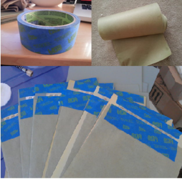
Figure 6 – Top, masking paper and scotch blue#2093EL. Bottom, stencil covered by masking paper and scotch blue#2093EL on Al panel.
