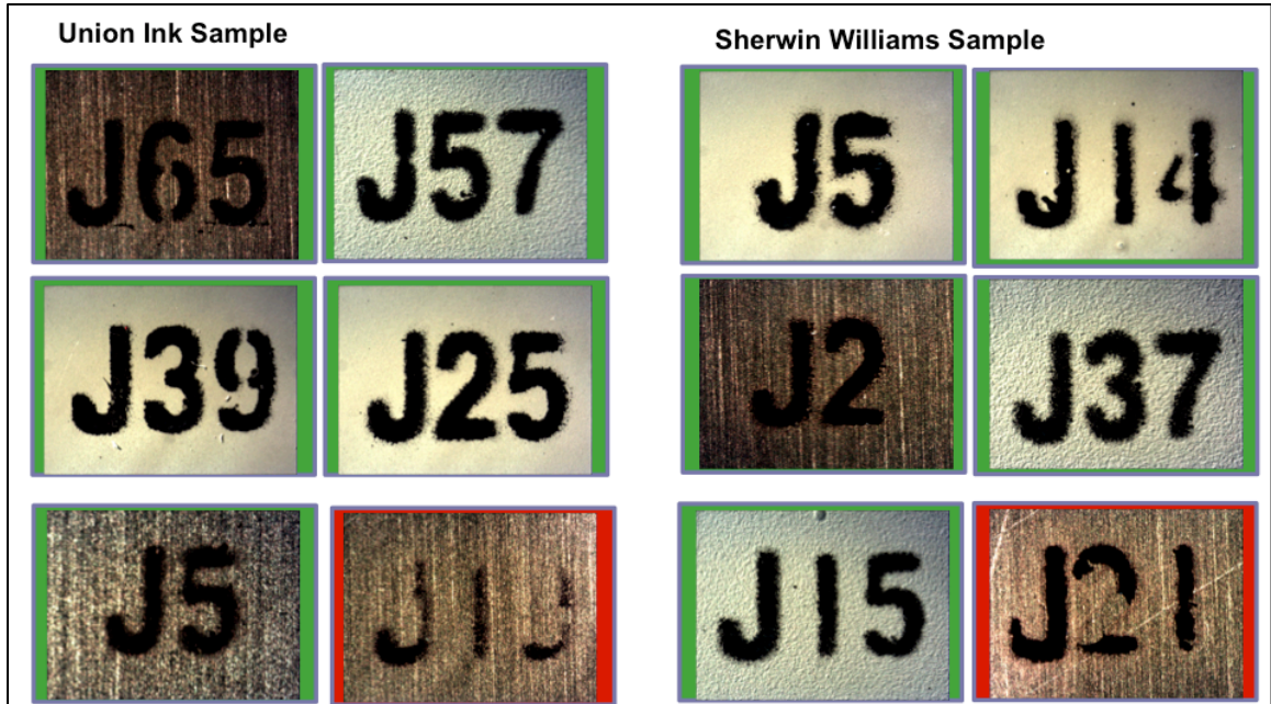
Figure 13 - Snapshot of 10x magnification of Cleaning Systems Test of Union Ink and Sherwin Williams samples.
