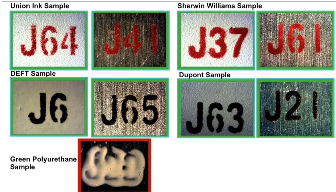
Figure 9 - Snapshot of 10x magnification of Thermal Shock results
