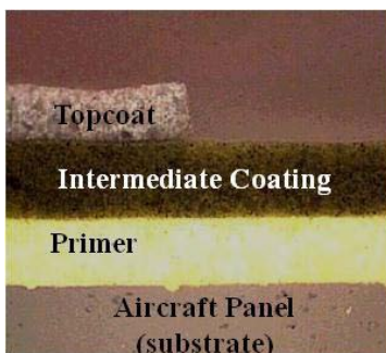
Figure 2 - Barrier coat encapsulating chrome primer. [3]
