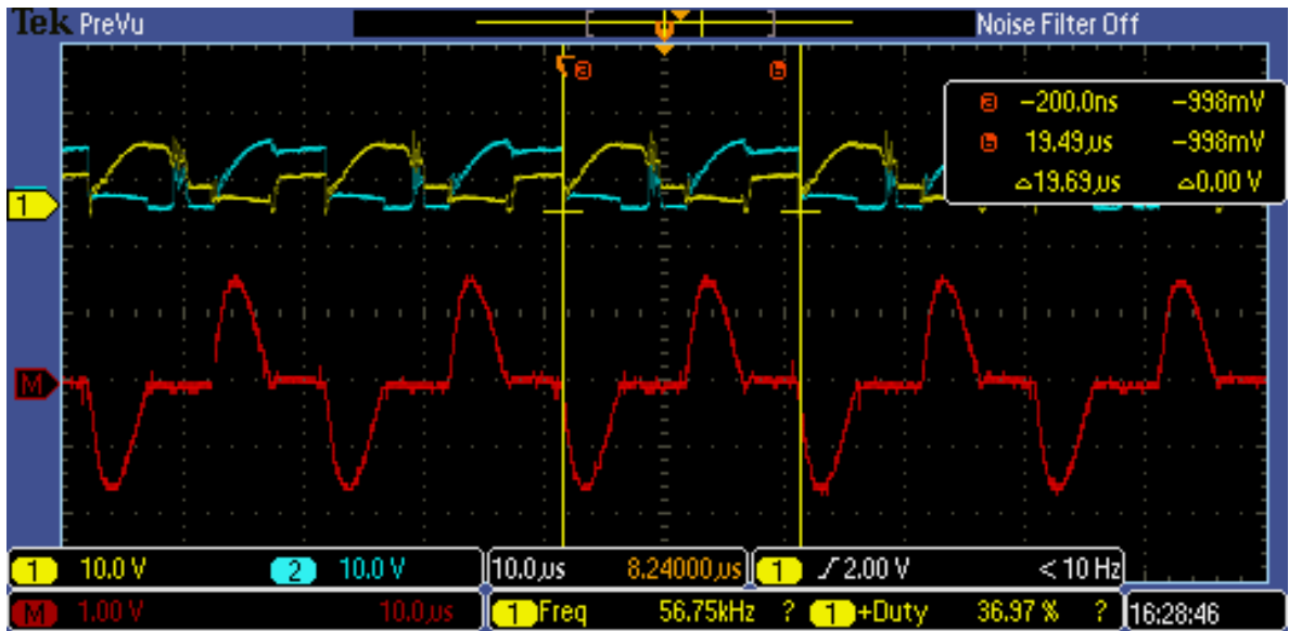
Figure 5.24: Result of the Arduino and bridge driver system, showing inductor current.
