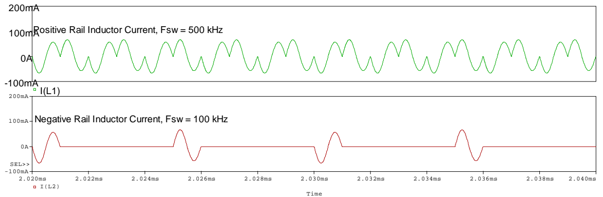
Figure 4.6: Positive rail remaining at BCM at 500kHz, Negative rail operating in DCM at 100kHz.
