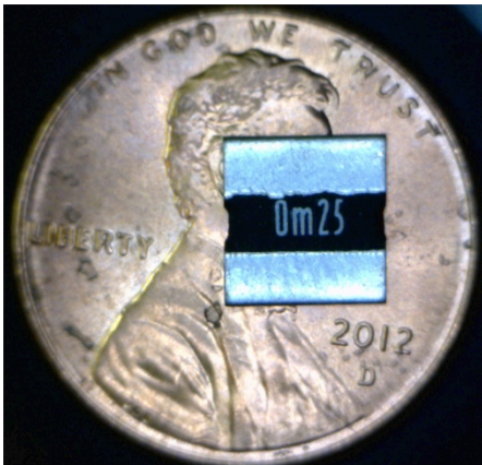
Figure 4.4 – 250\mu\Omega sense resistor (size 2725) on a penny.
