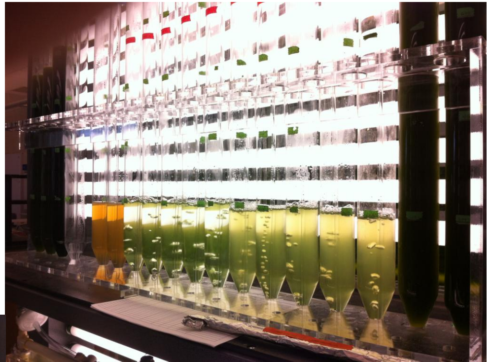
Figure 28 (Above): Photo showing light rack after inoculation of digestate regrowth experiment. From left to right: x3 Nannochloropsis maintenance cultures, x2 HTL, x5 controls, x5 digestate columns (50% v/v dilution), x2 Nannochloropsis maintenance cultures.
