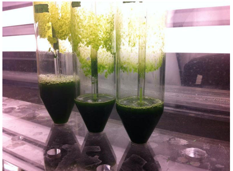
Figure 317: Photograph of the digestate columns on April 17, 2014. The columns gained the dark, green color after the addition of trace metals and micronutrients.
