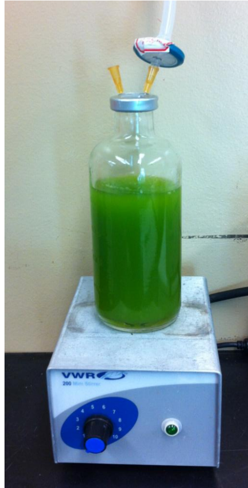
Figure 9: Carbon purging system for algae growth vessels. Culture was agitated using a stir plate while 100% CO 2 was pumped into the headspace through the sterile syringe filter. An oxygen and carbon dioxide mixture exited the growth vessel through the second sterile needle.
