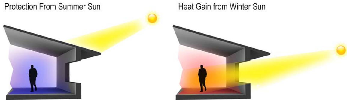
Figure 2.3.2: Solar Shade Diagram
