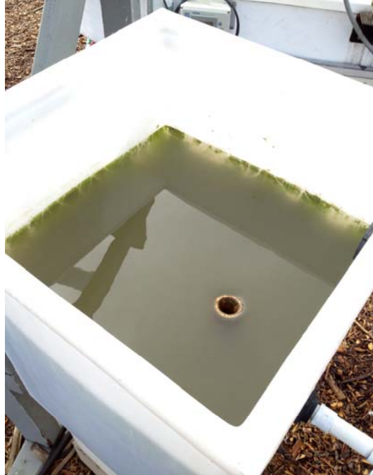
Figure 3.3: Primary treated wastewater constant head tank distribution system. Water level maintained at 48 cm (75% of tank height) using standpipe. Flow rate held constant throughout the experiment
