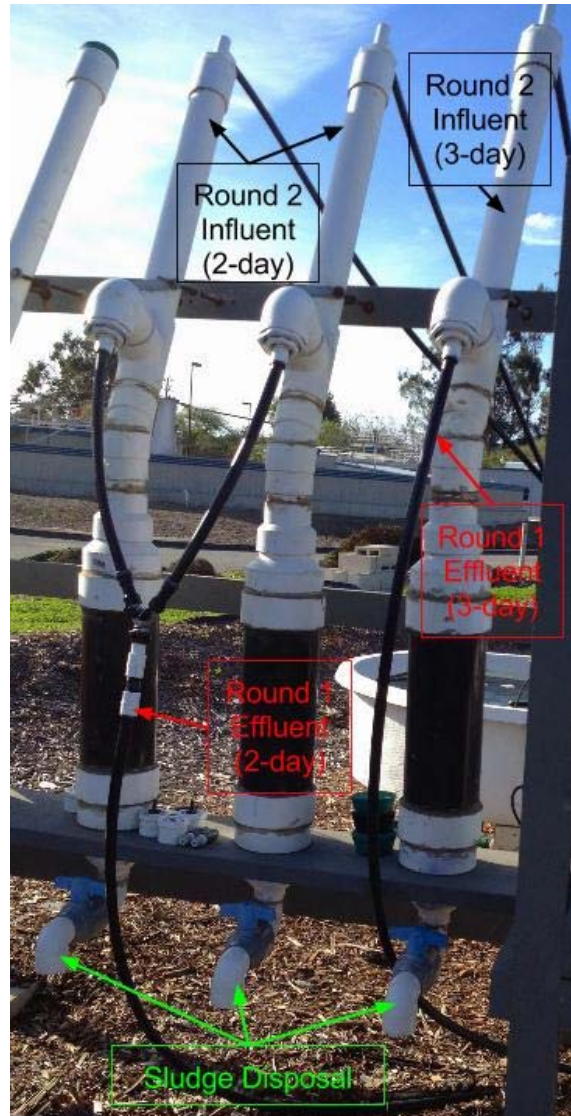
Figure 3.6: Tube settlers were positioned near the Round 2 ponds for convenience and minimal tubing
