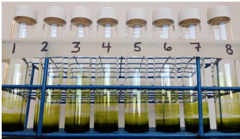
Figure 3.13: Lipid content was a dried residue in the vials after solvent was evaporated.
