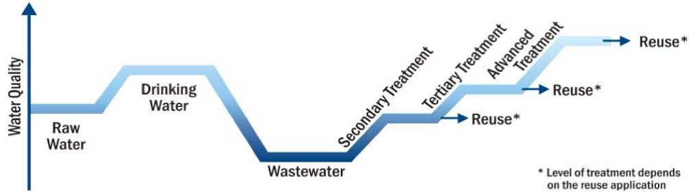
Figure 2.4: Water quality of recycled water depends on the level of wastewater treatment (EPA, 2012)
