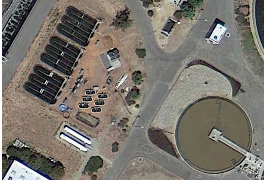
Figure 3.1: Aerial view of algae ponds (left) on-site near the primary clarifier (right)
