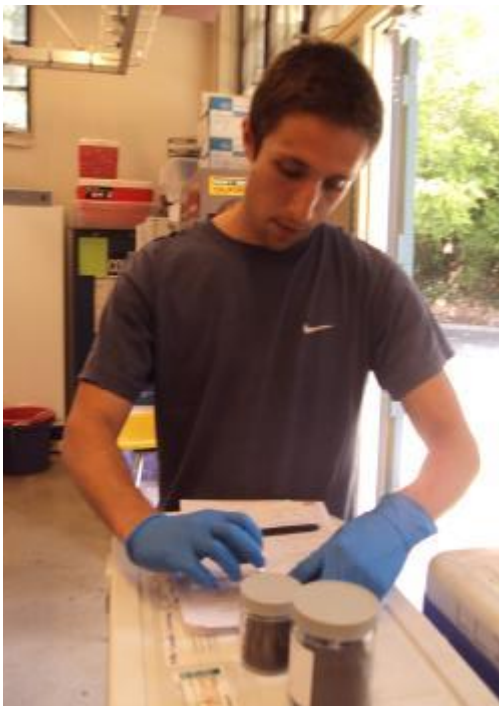
Figure 6: Soil sample processing: labeling and completing the chain of custody
