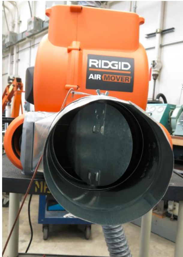
Figure 48. Air mover with butterfly valve and ducting for temperature control
