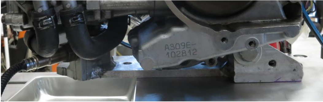
Figure 12. One piece aluminum engine mount
