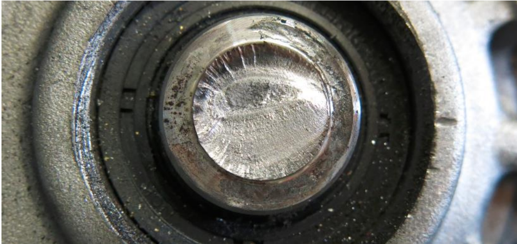
Figure 45. Crankshaft failure plane on output side
