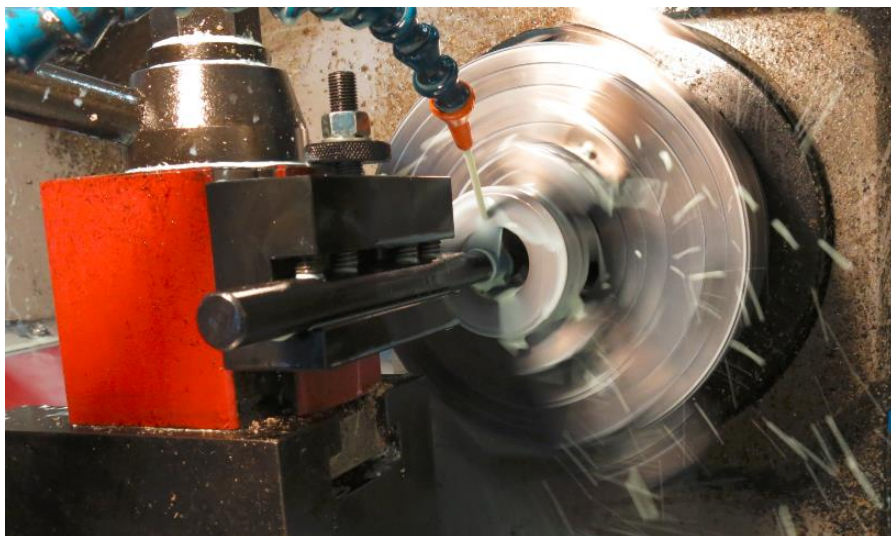
Figure 16. Boring of 32mm coupler
