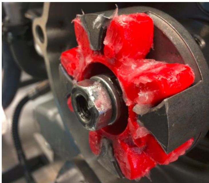
Figure 53. Stiffer elastomer installed with lubrication
