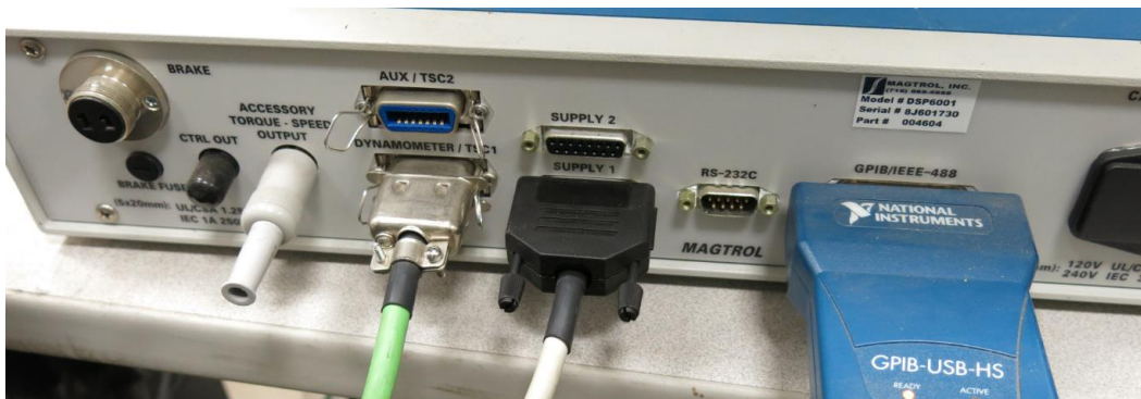
Figure 7. Connections on the DSP 6001 Controller
