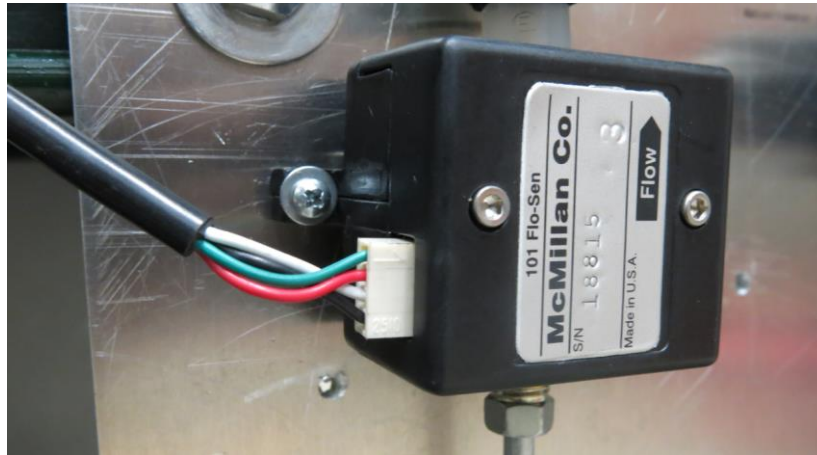
Figure 25. McMillan Model 101 20-100 mL flowmeter implemented on dynamometer
