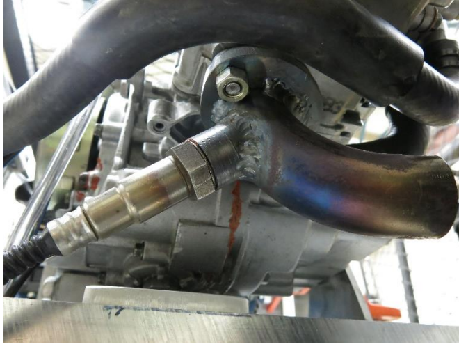
Figure 14. Revised steel exhaust runner
