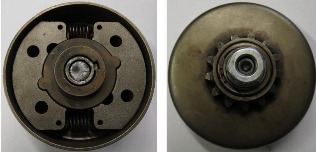
Figure 89. Centrifugal clutch used in prototype vehicle
