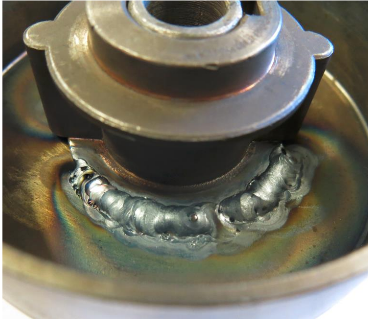
Figure 44. Welded centrifugal clutch
