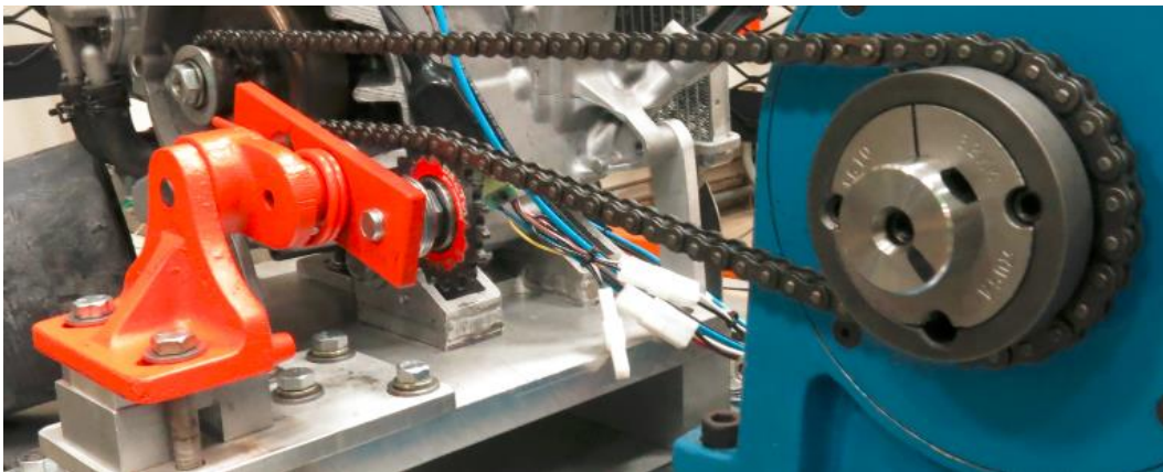
Figure 46. Torsion spring tensioner setup
