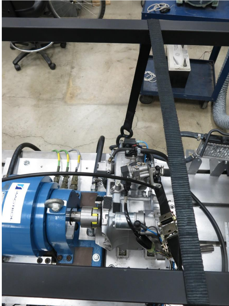
Figure 19. Supporting ratchet strap used to assist in coupler alignment
