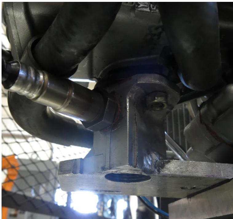
Figure 13. Existing mount and exhaust
