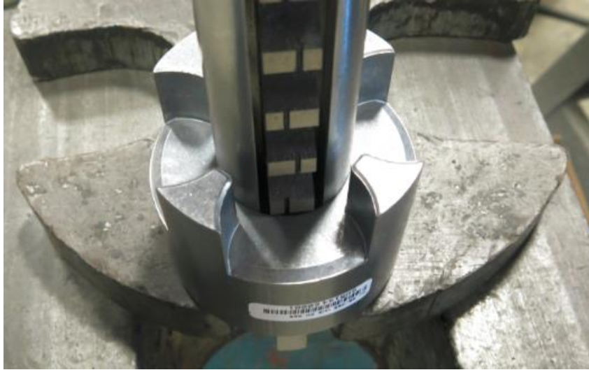
Figure 17. Broaching of 10mm key for 32mm coupler
