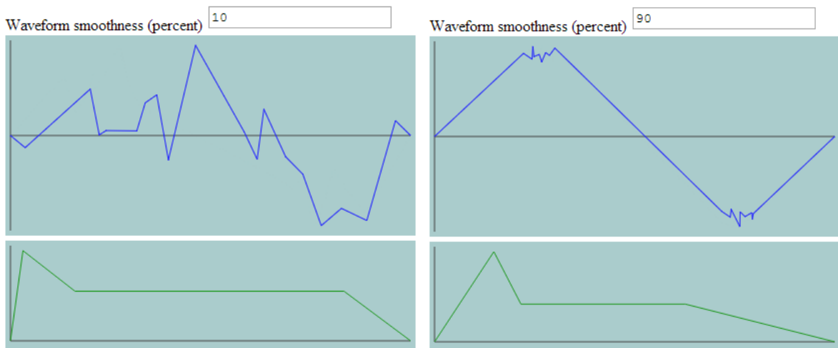
Figure 4.3: AUD.js uses randomized waveforms with a smoothness factor tied to the stress level, and randomized ASDR envelopes.
