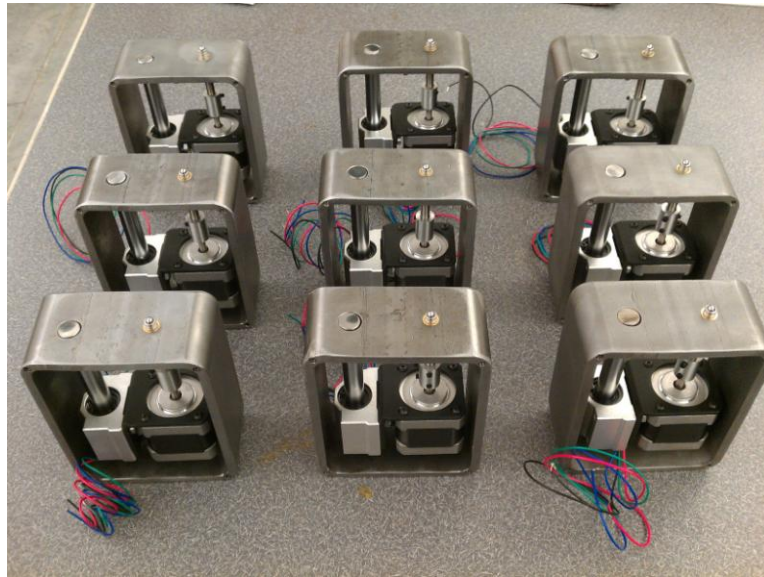
Figure 12: Actuators before side covers and paint
