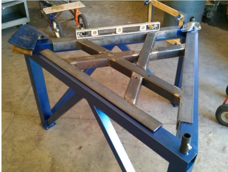
Figure 11: Mirror support frame being test fit onto telescope base
