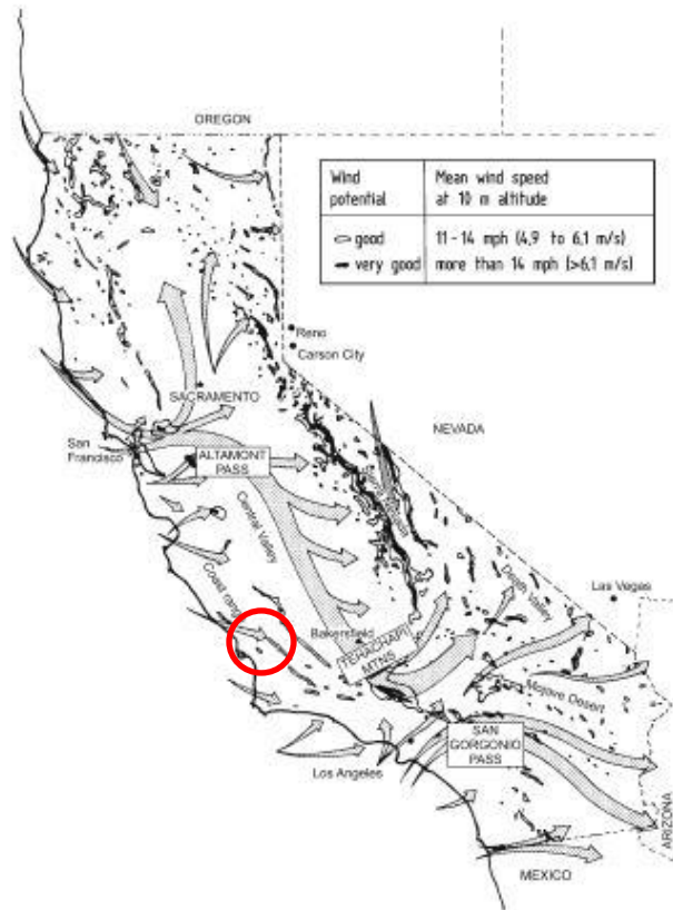
Figure 1 Wind speed magnitude at an altitude of 10 meters denoted by arrow size for California, San Luis Obispo circled in red.
