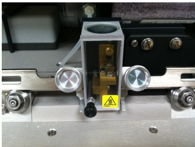
Figure 11.3 Image of glass pipette pushed towards the left and secured by both knobs
