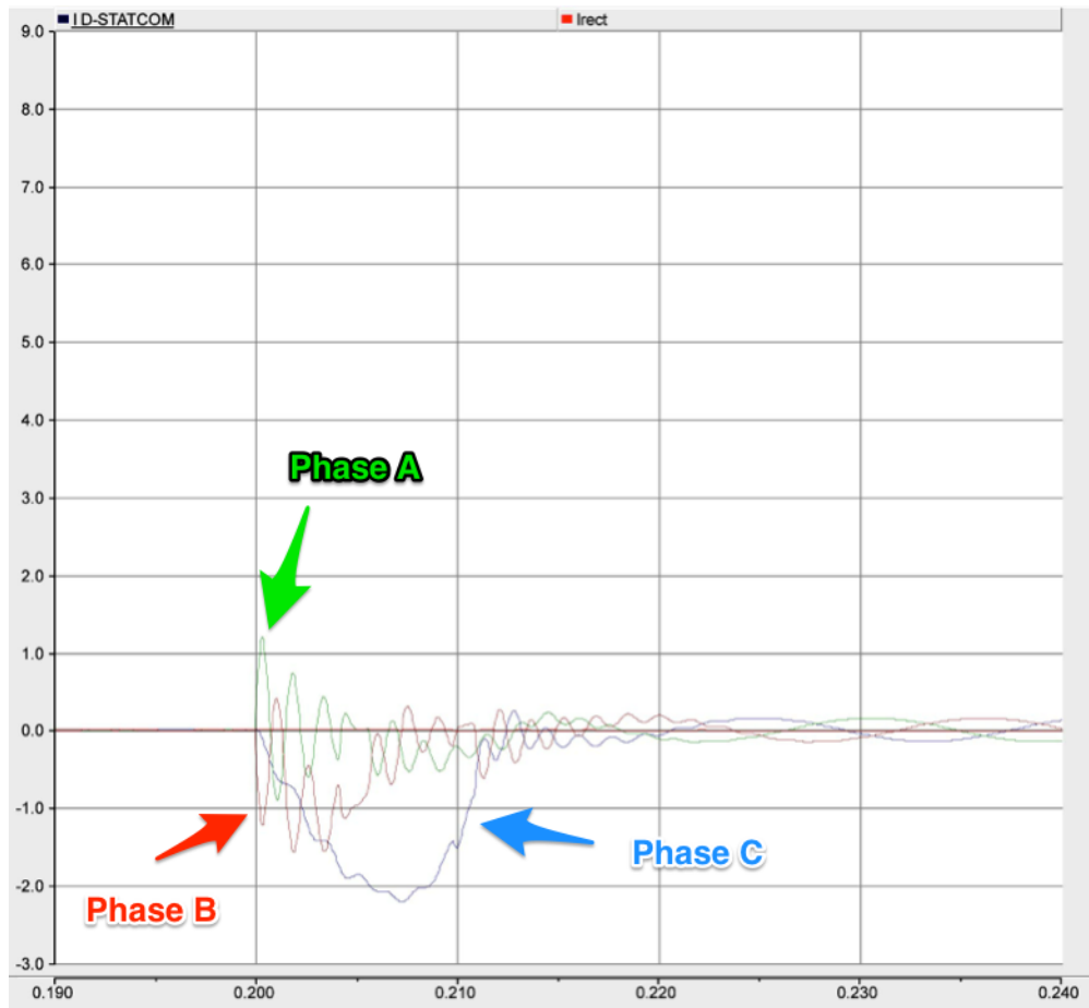
Figure 5.3 Inrush Current, Single Operation without Parallel Rectifier
