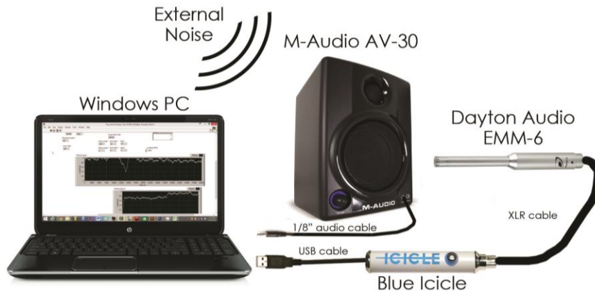
Figure 5-16: Complete system test-setup with external noise source.
