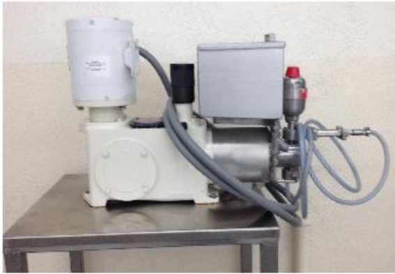
Cleextral Super K PP8 Diaphragm Pump Output: up to 8 l/h Flow adjustable from 0 to 100 %
