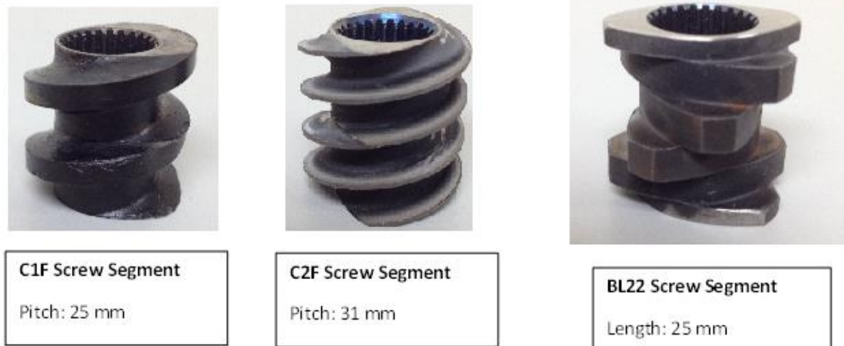
Figure 3.4 Screw segments used in screw profile design (Source: Cleextral Inc.)
