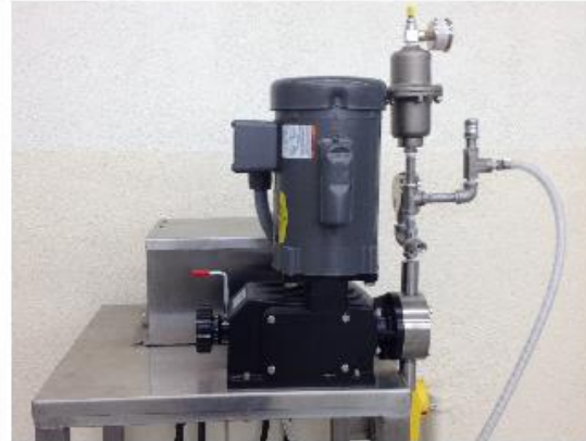
Novatech OMNI DC2A2AP Metering Pump Output: up to 26 l/h Flow adjustable from 0 to 100 %
