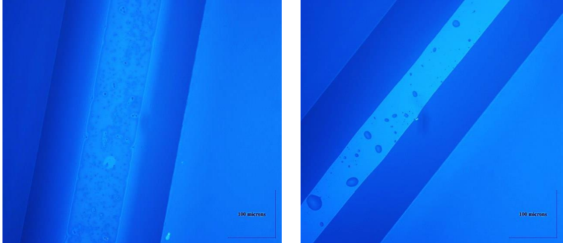
Figure 28. Effect of wetting agent on bubble in channel. Left: Channel bubble with wetting solution. Right: Channel bubble without wetting solution.
