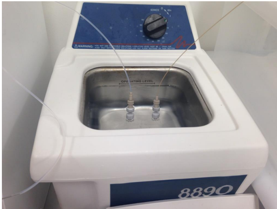
Figure 26. Translume channel cleaning. Translume channel suspended in sonic bath to remove particles stuck to channel walls.
