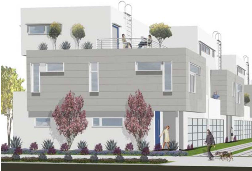
Architectural rendering highlighting roof gardens, entry ways and grasscrete driveway. Also note the visual interest created by the use of materials and varied window orientation.
