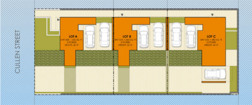
Site plan shows linear configuration with a shared driveway and a pedestrian path separate from driveway.
