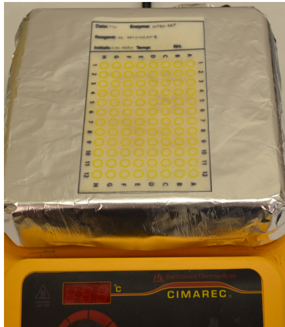
Figure 2.2.5.: Post and hard bake setup for microPAD.
