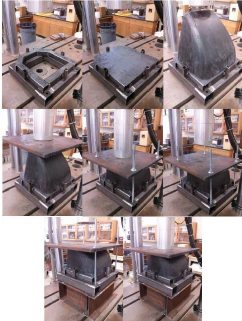
Figure 8: Test procedure, from setup to end of test. A mid-test change to account for lack of piston travel is shown. This change occurs at 145 mm of displacement.
