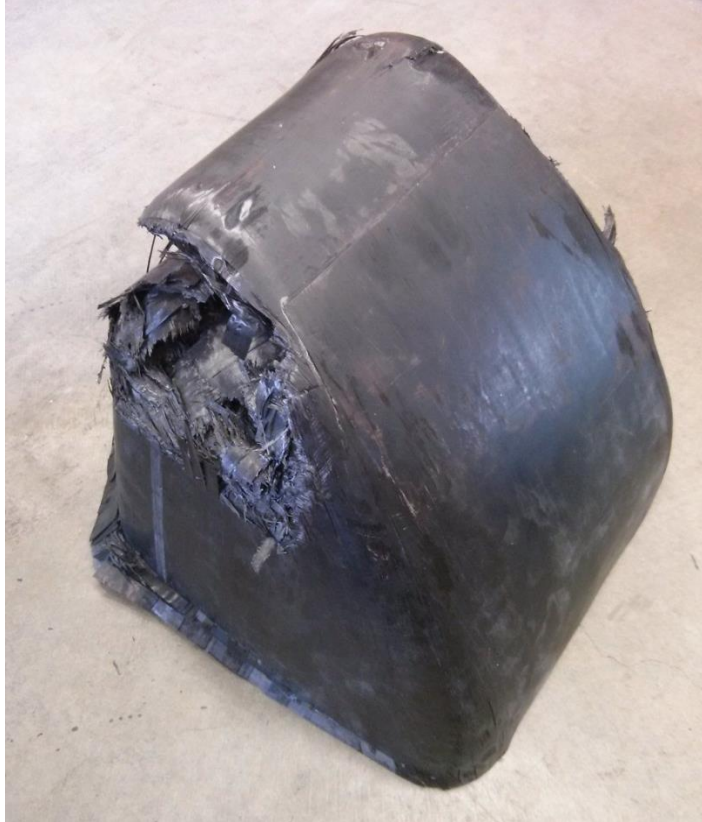
Figure 5-5 – Nosecone post quasi-static crush test.
