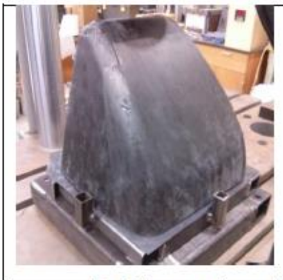
Figure 3: Attenuator as Constructed
