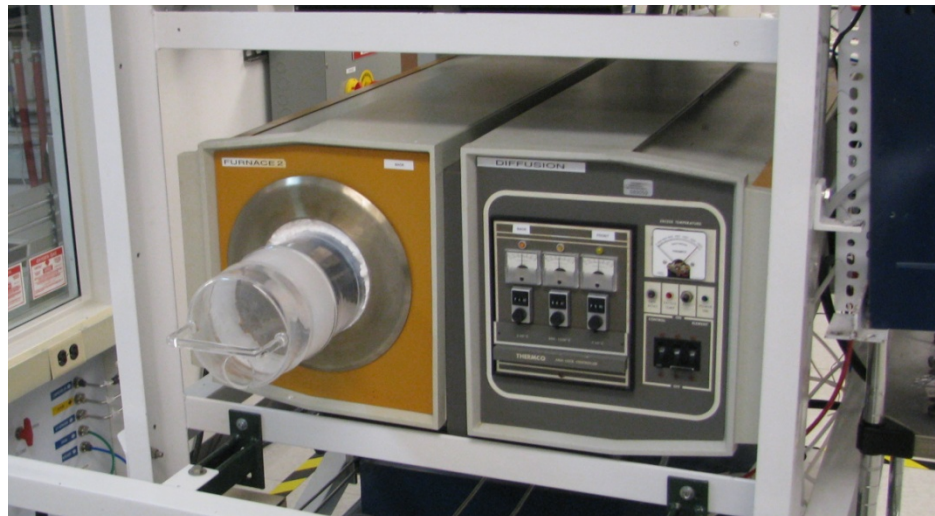
Figure 14: Thermal oxidation furnace in Cal Poly Microfabrication Lab.
