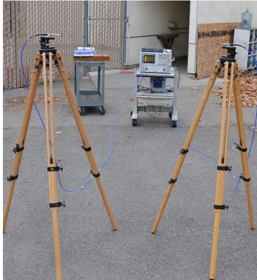
Figure 22: S_{21} measurement test configuration. DUT spacing and orientation is carefully controlled for repeatable measurements. Non-reflective wooden tripods are used to reduce interference.
