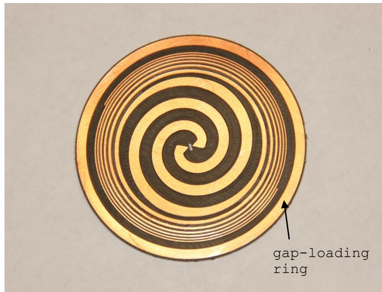
Figure 14: Combination spiral with gap-loading ring. Gap-loading is a space-efficient method of reducing antenna cutoff frequency.
