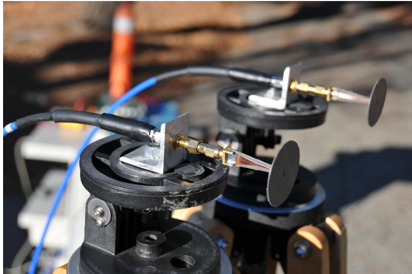
Figure 27: Cross coupling measurement test configuration. Spacing is the minimum capable while mounted on the tripods.
