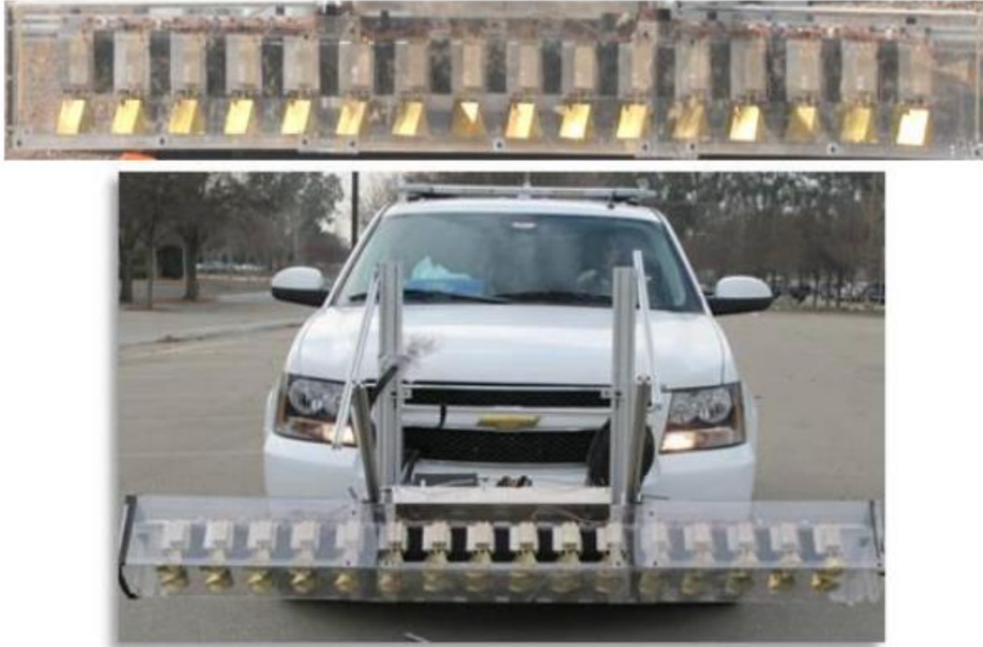
Figure 5: Top: 16-element ground-penetrating radar array. The antennas used in this example are hexagonal horn antennas. Bottom: Array mounted to an SUV for system testing.
