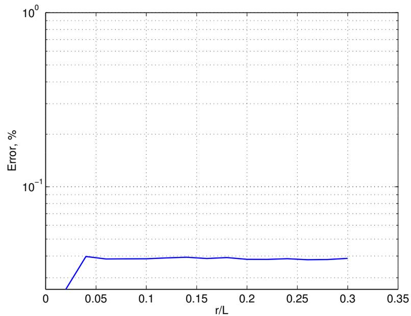
**Figure 8.3: Error on the drag results from the sweep of Sears-Haack bodies through the wave drag tool.**
