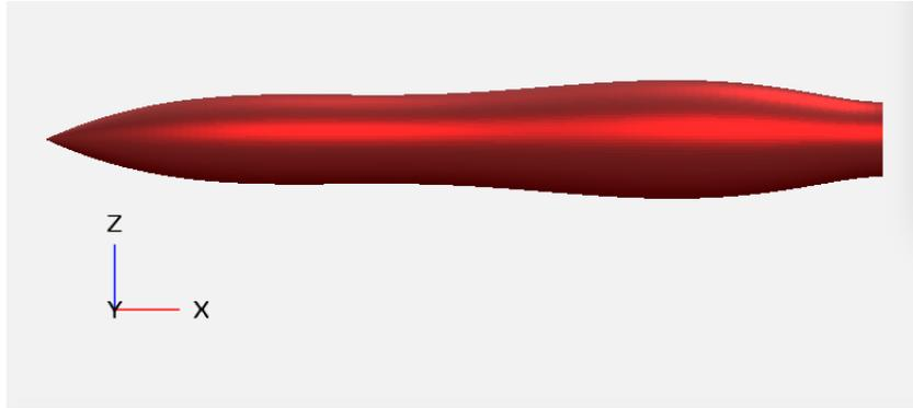
**Figure 8.7: OpenVSP model of an Eminton and Lord body ( $L = 40$ ) after being imported from a Hermite file.**
