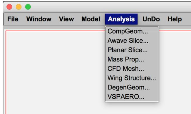
**Figure 2.3: The options contained within the Analysis tab of OpenVSP.**
