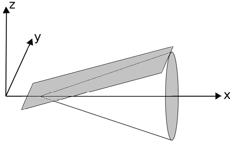
**Figure 3.2: A Mach plane corresponding to a given Mach cone.**
