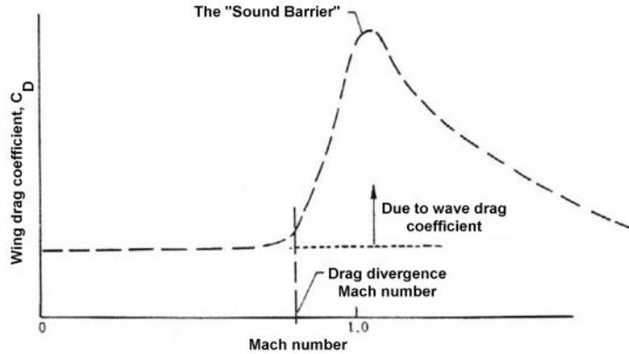
**Figure 1.1: Illustration of transonic drag rise [5].**
