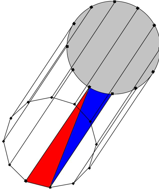
**Figure 5.13: Depiction of triangles added after translating copies of subsurface intersection nodes. The red and blue triangles highlight how each rectangle of four nodes becomes two meshed triangles.**
