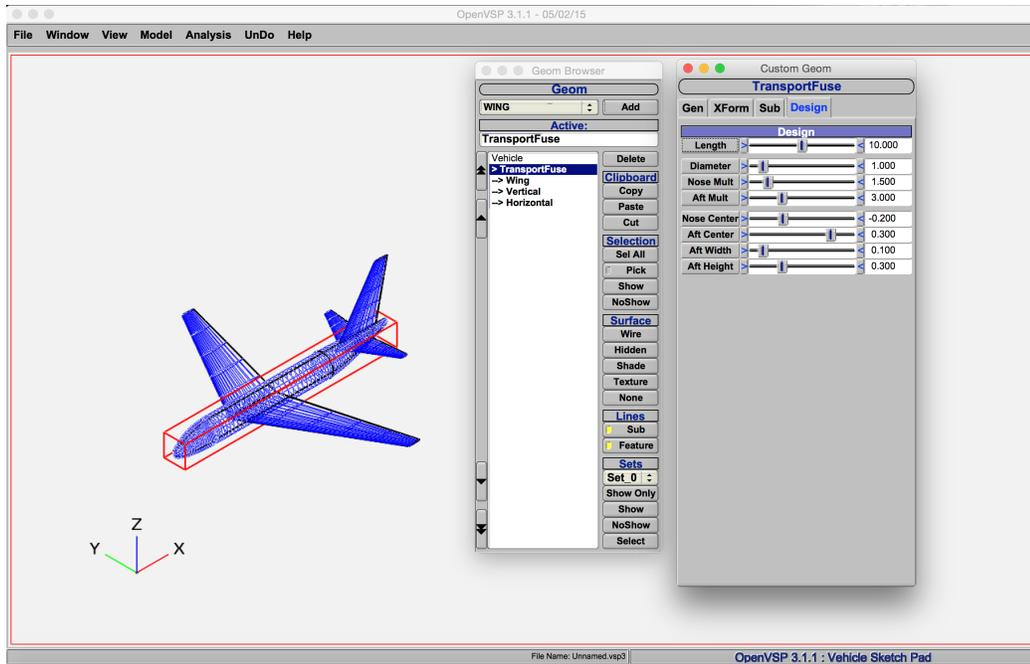
**Figure 2.2: OpenVSP home screen, showing example transport model with geometry user interfaces.**
