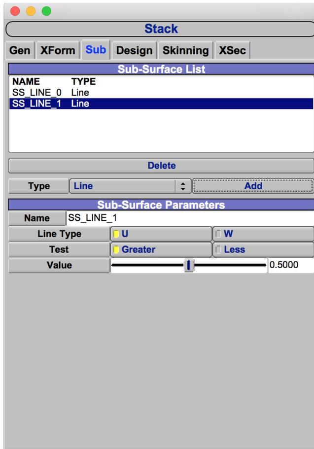
**Figure 7.5: Subsurface tab on a stack component.**
