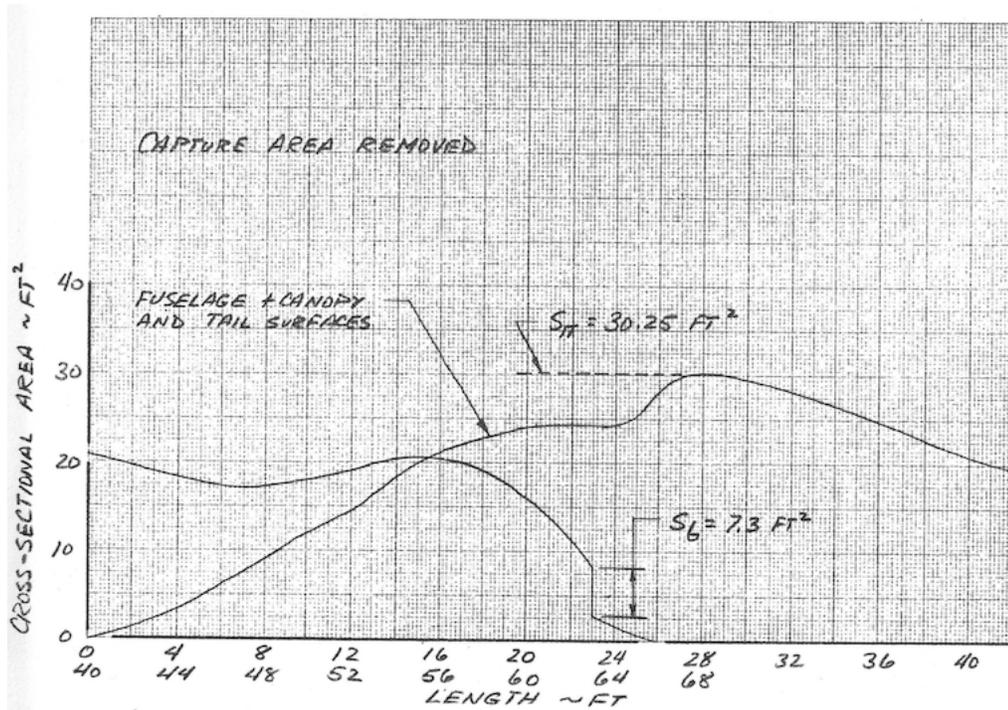
Figure 4.9: Cross-sectional area distribution for the F-106A [24]. Here, capture area has been removed.
