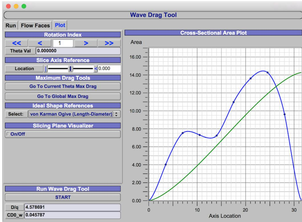
**Figure 7.9: Overlay of the equivalent von Kármán body cross-sectional area curve selected in the fight model working example.**
