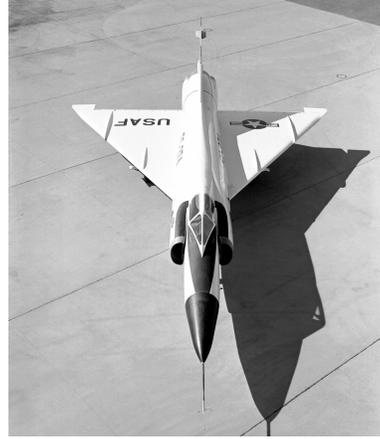
(b) The F-102A with area-ruled fuselage, necked down in the region of the wing.
