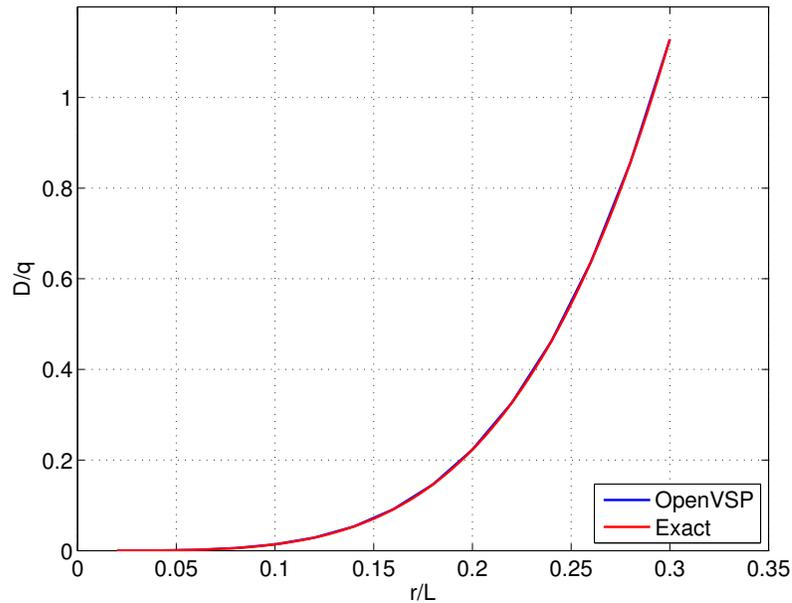
**Figure 8.2: Drag results from a sweep of Sears-Haack bodies through the wave drag tool compared to the analytical solution.**
