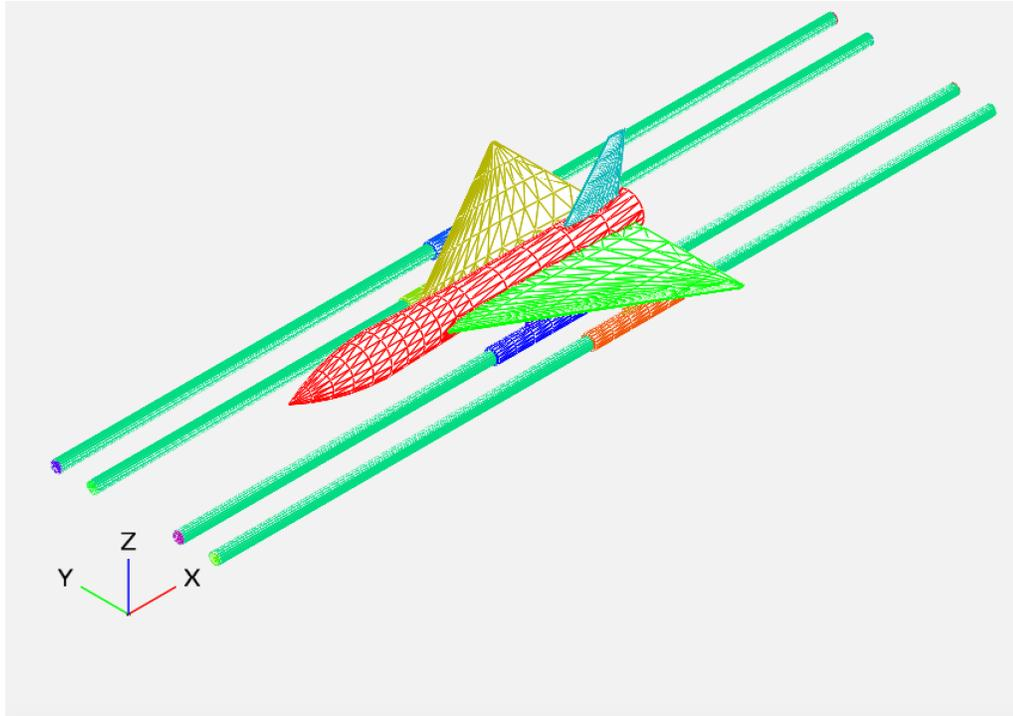
**Figure 5.14: Fighter example, showing extension of flow-through tubes after running the wave drag tool.**
