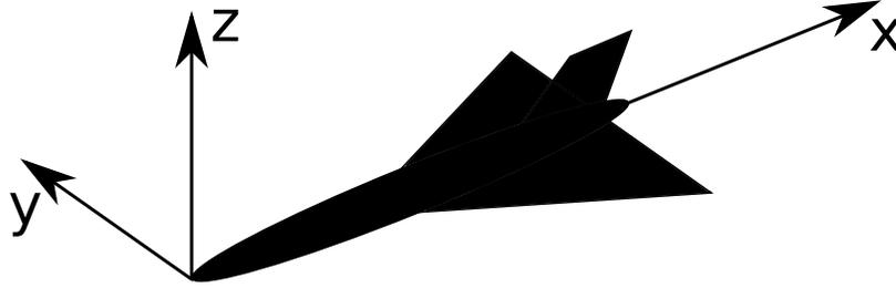
**Figure 3.4: Depiction of aircraft axis system used by OpenVSP.**
