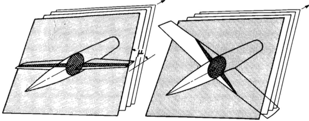
**Figure 3.3: Projected areas of Mach angle cutting planes intersecting a body [21].**
