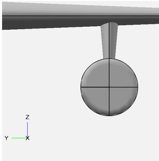
**Figure 5.7: Example fighter model engine component before inlet flow face subsurface has been added.**
