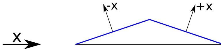
**Figure 5.12: Depiction of ambiguous subsurface norm  $x$ -components. The blue surface indicates the single face that points in two  $x$ -directions.**
