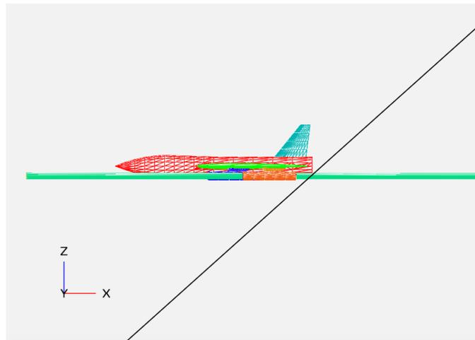
**Figure 5.16: Black line depicts Mach 1.5 cutting plane at slicing end location, with engine component inlet extension tubes extending aft of the slicing bound.**
