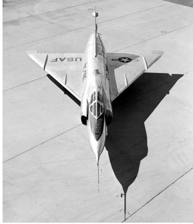
(a) The F-102 with straight fuselage.
