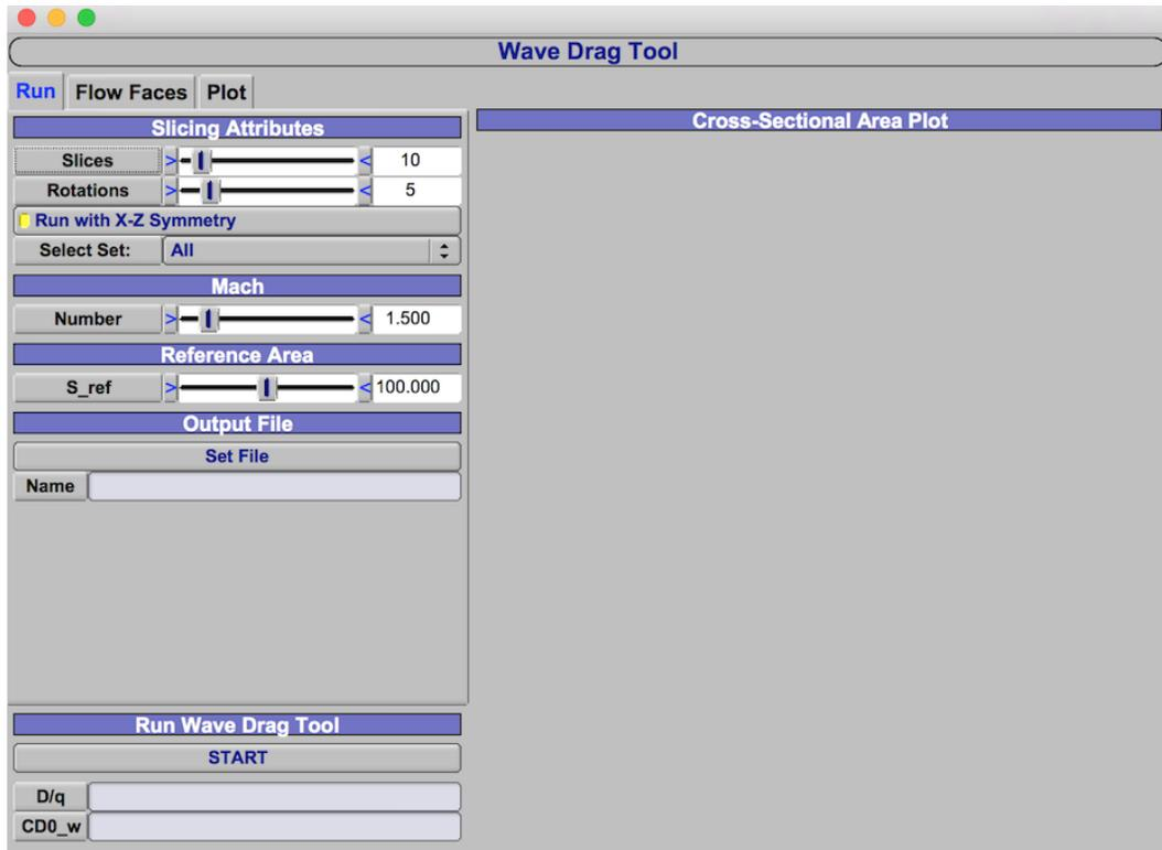
**Figure 7.2: Default wave drag tool GUI.**
