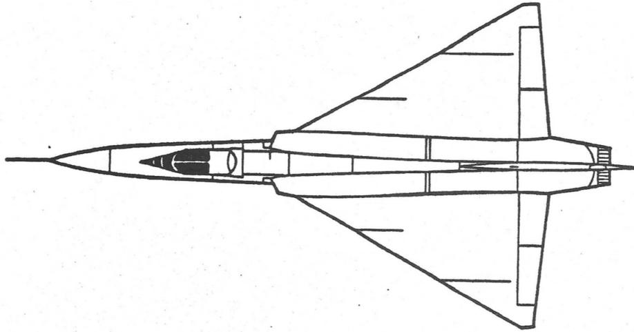
Figure 4.8: Top view drawing of an F-106A [24].
