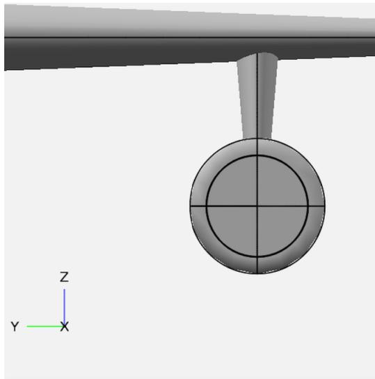
**Figure 5.8: Example fighter model engine component after inlet flow face subsurface has been added.**
