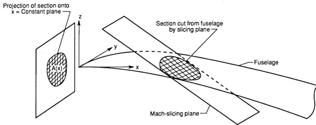
**Figure 5.5: Depiction of the projected area of a Mach cutting plane when intersected with a body [26].**
