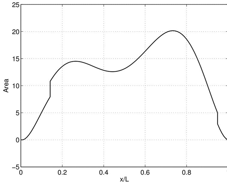
**Figure 4.4: Representative cross-sectional area distribution for the example in Figure 4.3.**
