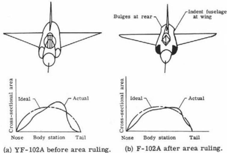
**Figure 1.3: Cross-sectional area distributions of the YF-102 and YF-102A [8].**
