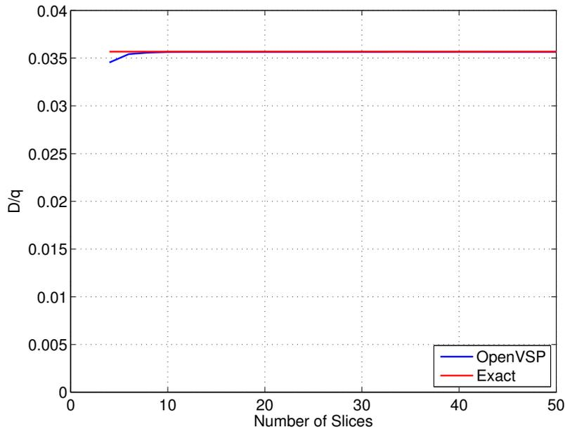
**Figure 8.5: Convergence study on the number of Mach cutting plane slices versus the wave drag result compared to the analytical solution for the Sears-Haack body.**
