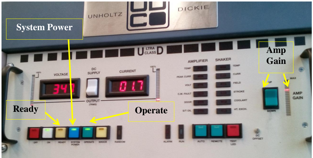
Figure 25: Buttons that operate the amplifier for the vibration table and experiments.
