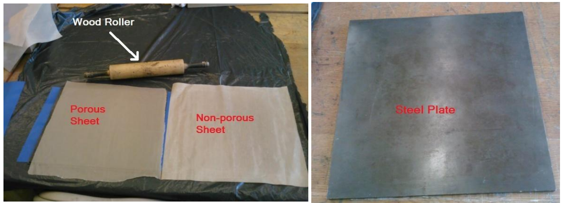
Figure 6: Lay-up for the pre-curing process of the composite plate.
