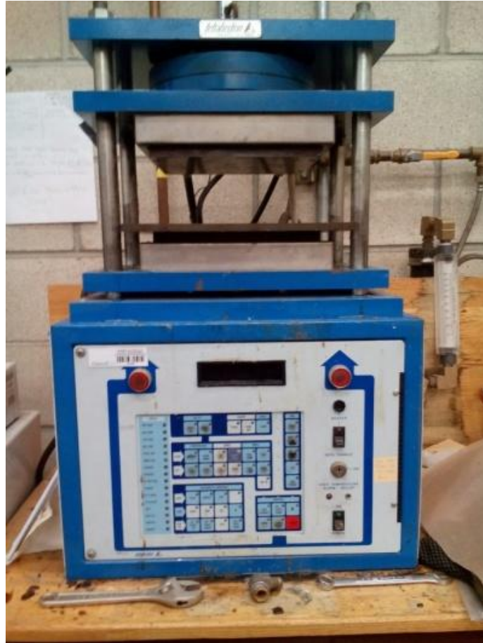
Figure 5: Press table where composite plate was cured.
