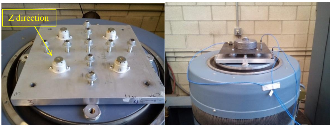
Figure 24: The z direction orientation for all isolator groups and test setup.
