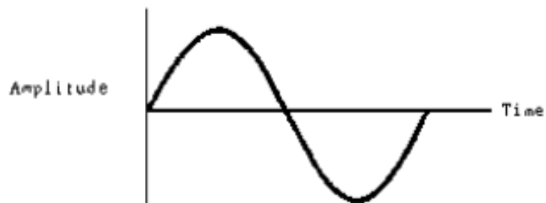
Figure 2: Amplitude and time history of sinusoidal vibration. [8]
