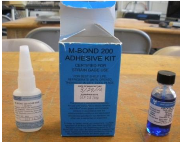
Figure 12: Chemical components used to connect strain gages to carbon fiber test samples.
