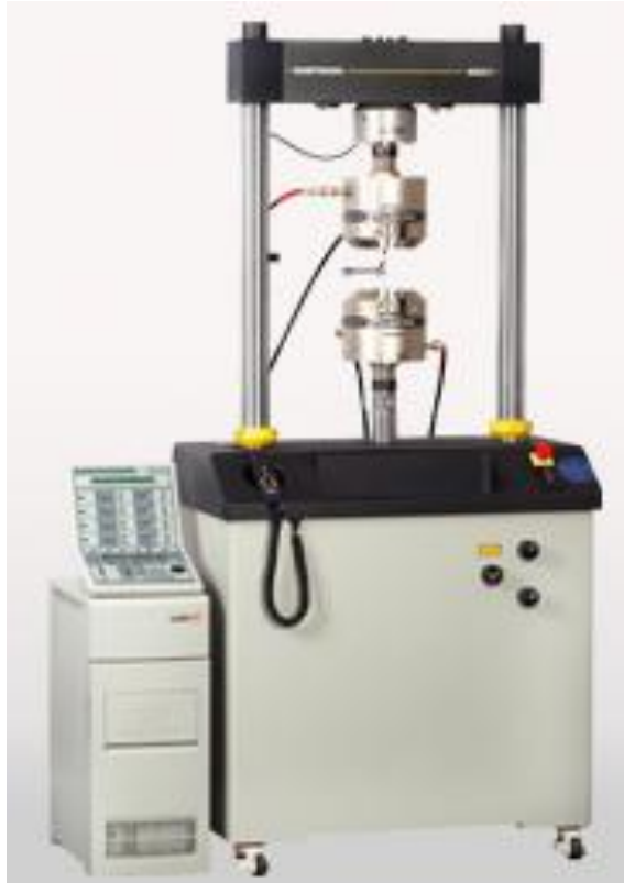
Figure 7: Instron machine utilized to acquire material properties of the carbon fiber composite plate.
