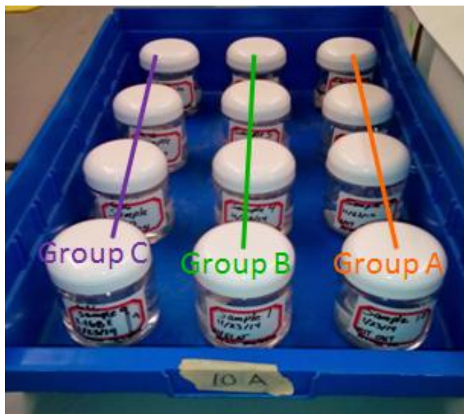
Figure 44: Twelve glass jars for different outgassing cases with silicone materials.
