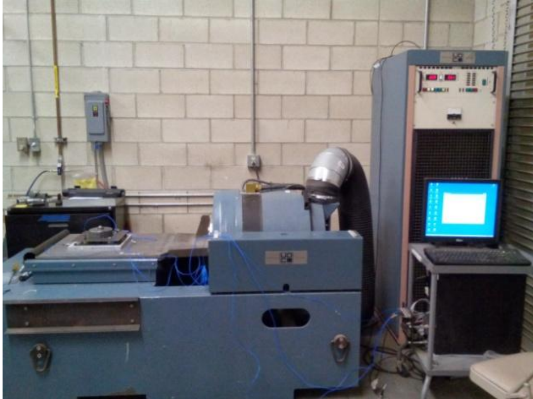
Figure 19: Vibration system used for the flat and high frequency energy spectrum tests.
