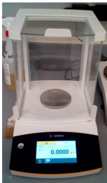
Figure 45: Sartorius high precision scale used to weight the silicone samples for swelling tests.
